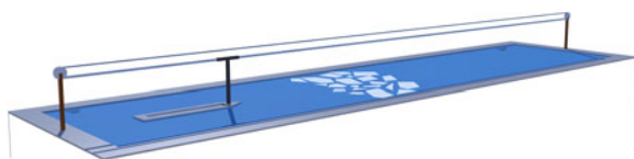
Fig. 14. Schematic experiment layout, showing the vessel, some floes and the towing carriage above the tank.
