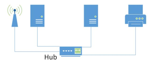
The set of hosts connected to the same hub is called an ethernet segment
