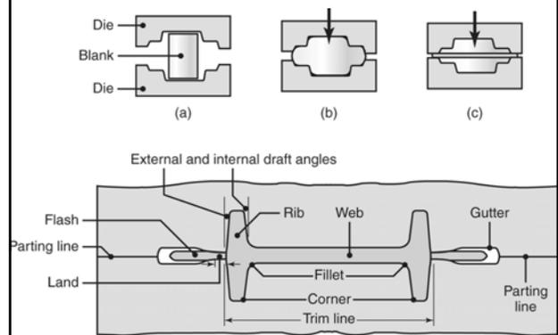
**FIGURE 14.6** Die inserts used in forging an automotive axle housing. (See Section 5.7 for die materials.)
