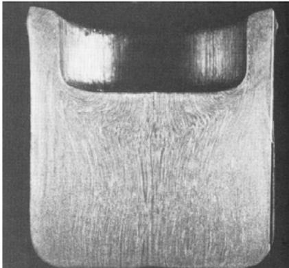
**FIGURE 14.13** (a) The stepped pin used in Case Study 14.1. (b) Illustration of the manufacturing steps used to produce the stepped pin. Source: Courtesy of National Machinery, LLC.
