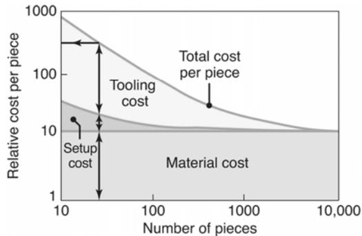
**FIGURE 14.19** Relative unit costs of a small connecting rod made by various forging and casting processes.
