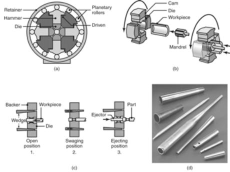
**FIGURE 14.15** (a) Swaging of tubes without a mandrel; note the increase in wall thickness in the die gap. (b) Swaging with a mandrel; note that the final wall thickness of the tube depends on the mandrel diameter. (c) Examples of cross sections of tubes produced by swaging on shaped mandrels. Rifling (internal spiral grooves) in small gun barrels can be made by this process.
