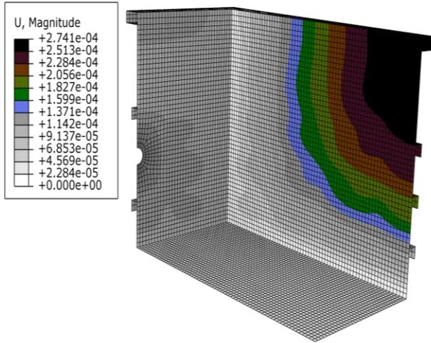
Figure 6. Deformation of test cell after gravity step.
