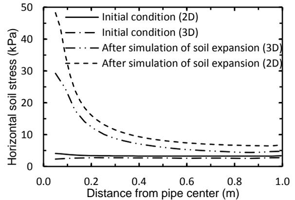
Figure 8. Horizontal soil stresses at springline level from pipe centre to cell wall.
