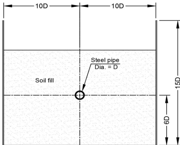
Figure 1. Schematic drawing of proposed test cell cross-section.
