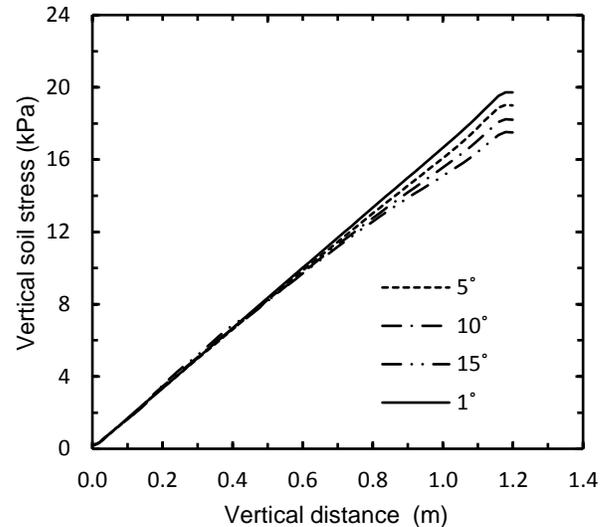
Figure 4. Vertical stresses with soil depth, 0.2 m away from the cell wall (initial loading).
