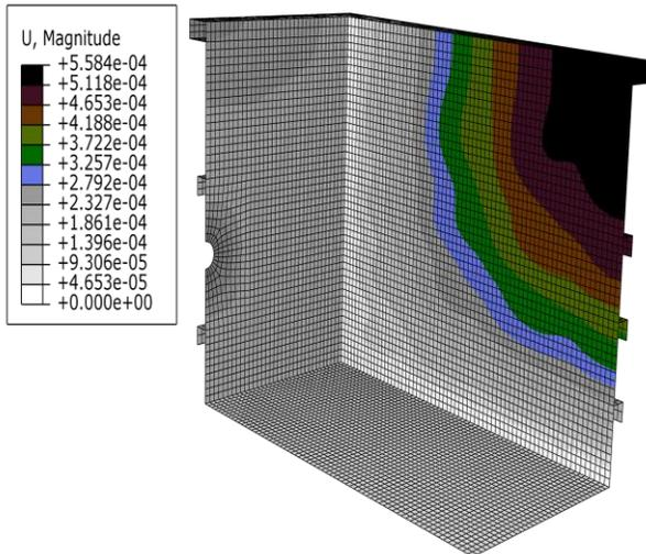
Figure 7. Deformation of test cell after simulation of dilation during the pullout.
