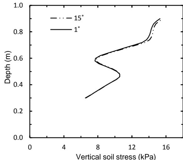
Figure 5. Vertical stresses with soil depth, 0.2 m away from the pipe centre during expansion.
