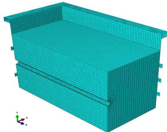
Figure 3. Typical finite-element mesh of soil, test cell and pipe used in 3-D model
