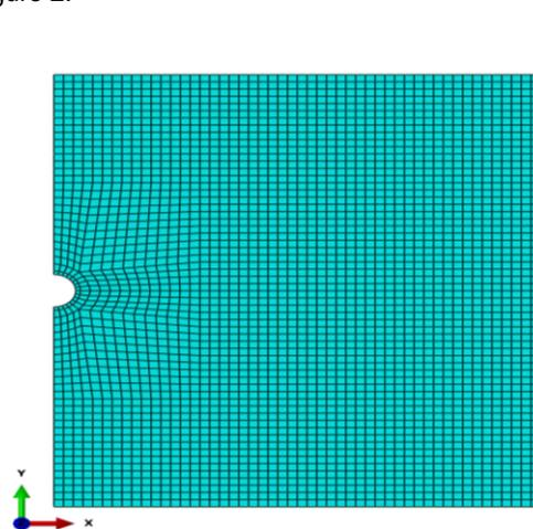
Figure 2. Typical finite-element mesh of soil, test cell and pipe used in 2-D model
