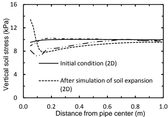
Figure 9. Vertical soil stresses at springline level from pipe centre to the cell wall.
