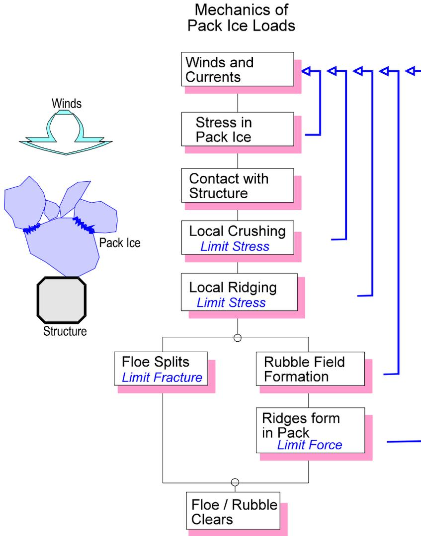
Figure 39. Conceptual Elements of Pack Ice-Structure Interaction
