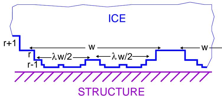
**Figure 15. Fractal Contact Geometry (Bhat, 1990)**
