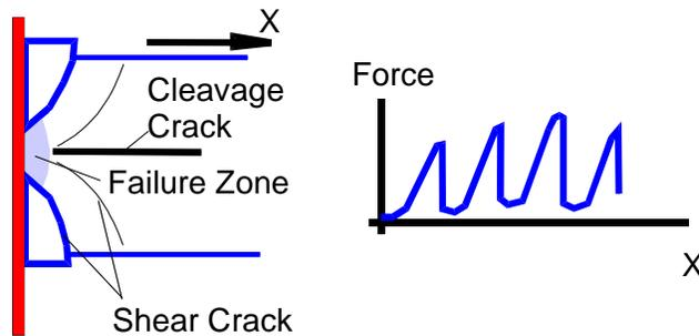
**Figure 8. Finite pulverization coupled with major shear flakes.**
