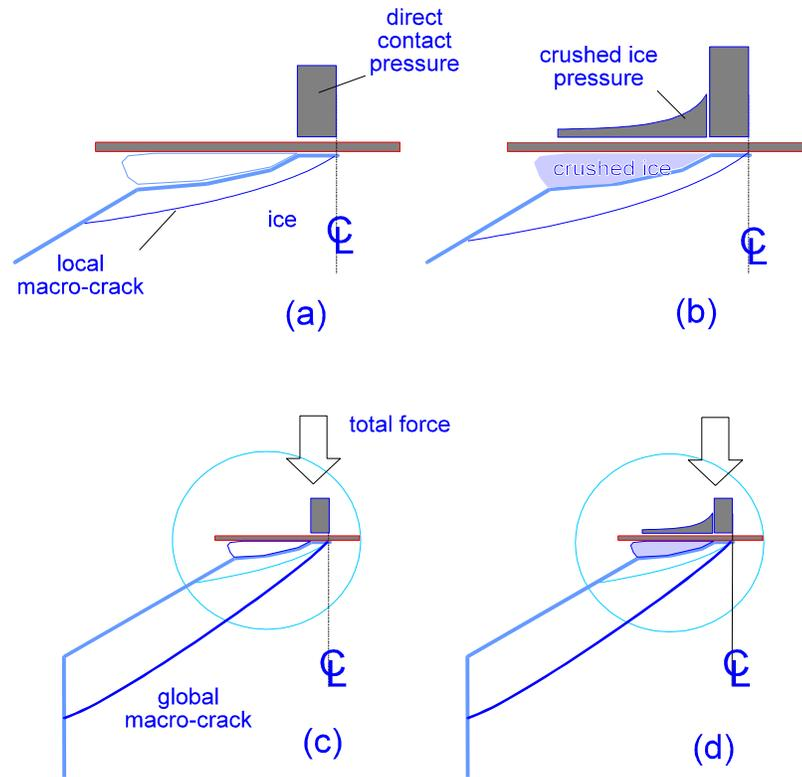
**Figure 42. Extrusion with Local and Global Flaking (Daley, 1992).**
