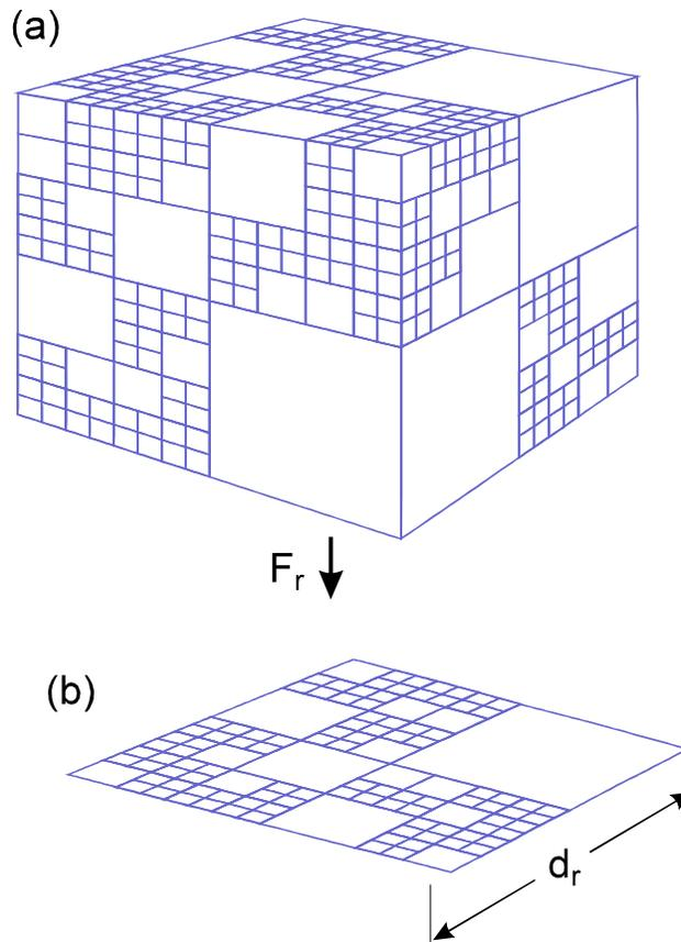
**Figure 16. Three dimensional fractal crushing of a brittle solid (Palmer and Sanderson, 1991).**
