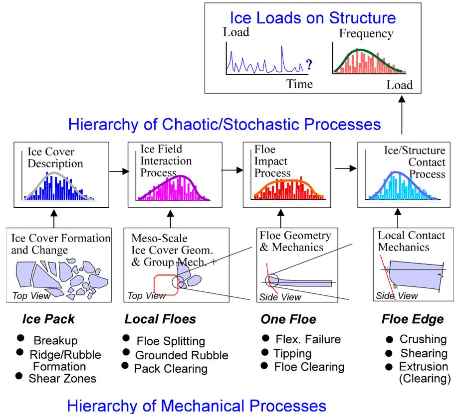
**Figure 2. Scales of Ice-Structure Interaction Mechanics**
