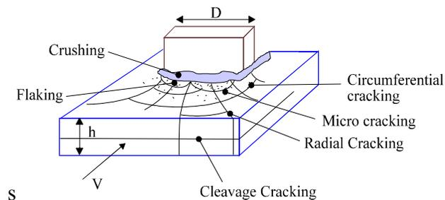
**Figure 10. Ice Failure Modes on a Vertical Structure (from Sodhi (1992) and Timco (1986))**
