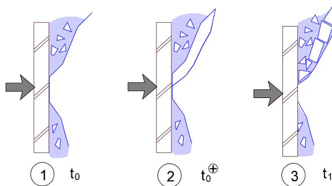
**Figure 27. Pulverization due to comminution of flakes created by macro cracks.**
