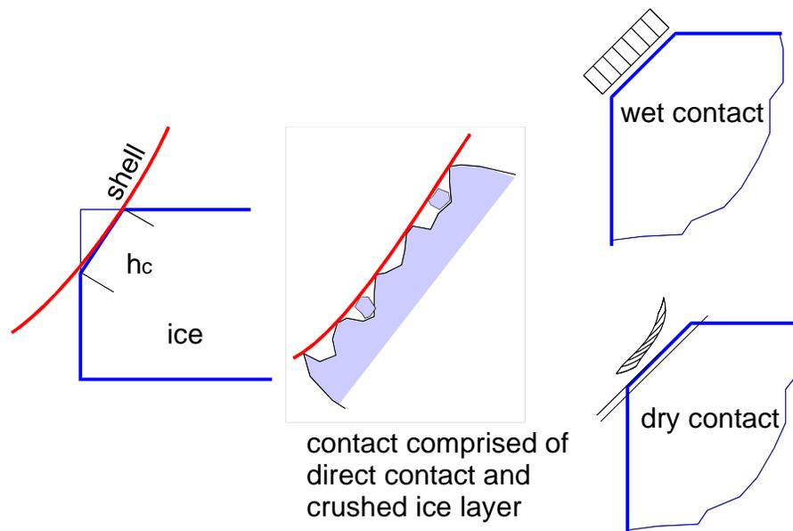
**Figure 5. Wet-dry contact model (Varsta, 1983).**
