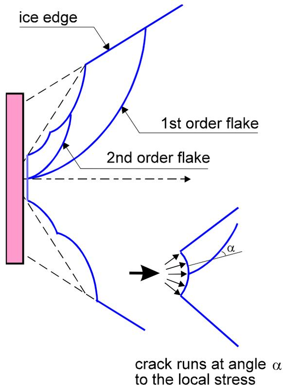
**Figure 24. Curved Flake Ice Load Model (Kujala, 1993 b)**
