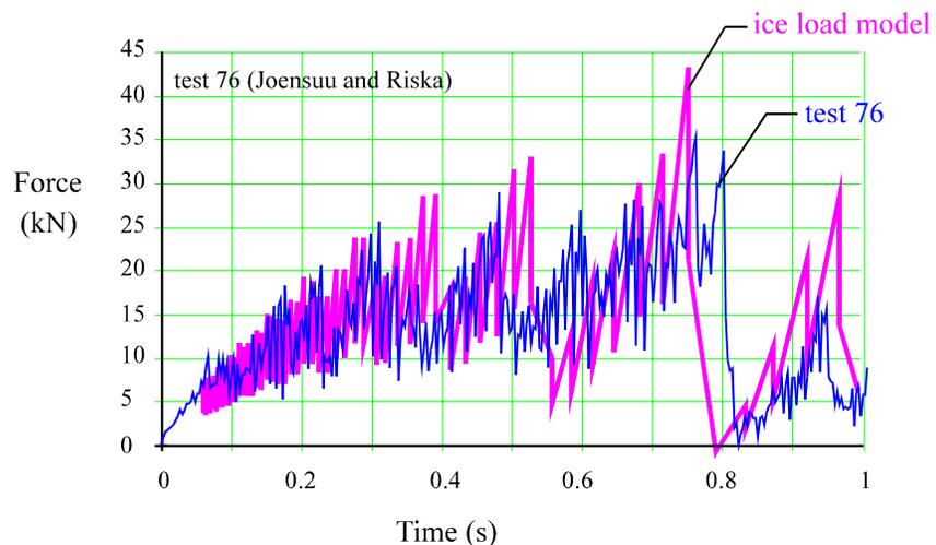
**Figure 23. Comparison of Joensuu-Riska test with ice load model (Daley 1991)**
