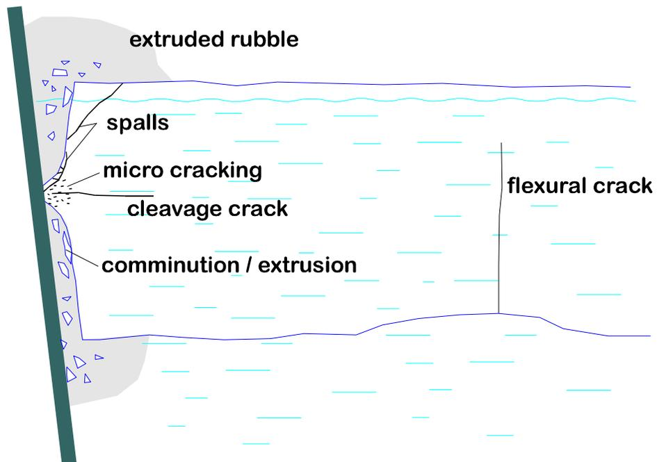
**Figure 29. Ice-structure contact showing various and simultaneous breakage mechanisms.**
