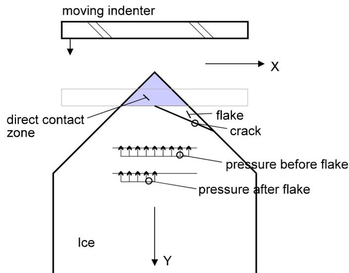
Figure 21. Mechanics of Contact Model (Daley 1990)
