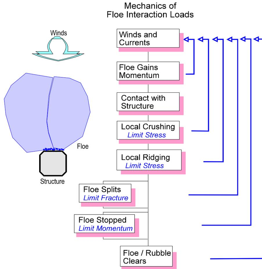
**Figure 38. Conceptual Elements of Floe-Structure Interaction**
