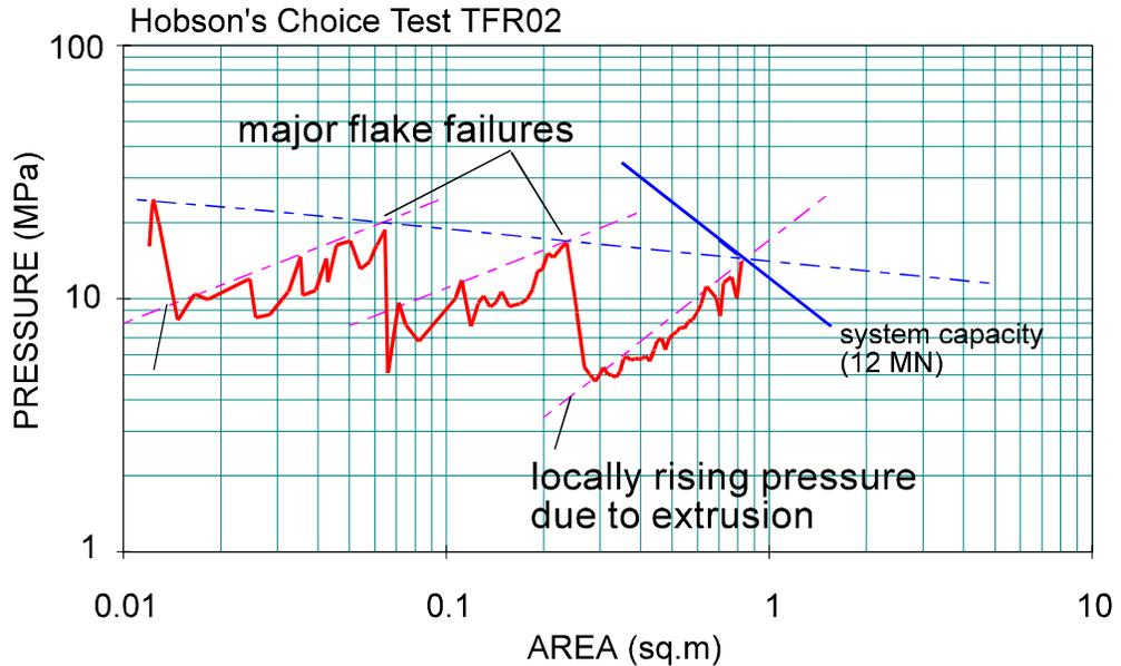
**Figure 41. Hobson's Choice Data Showing Discrete Failures (Daley, 1994)**
