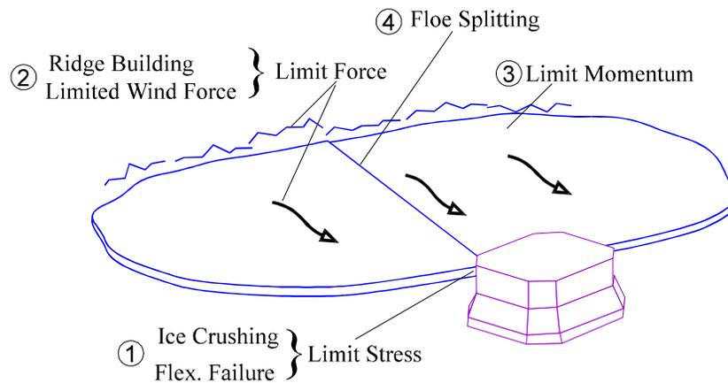
**Figure 34. Load Limits in Global Ice-Structure Interactions (modified from Croasdale 1984)**
