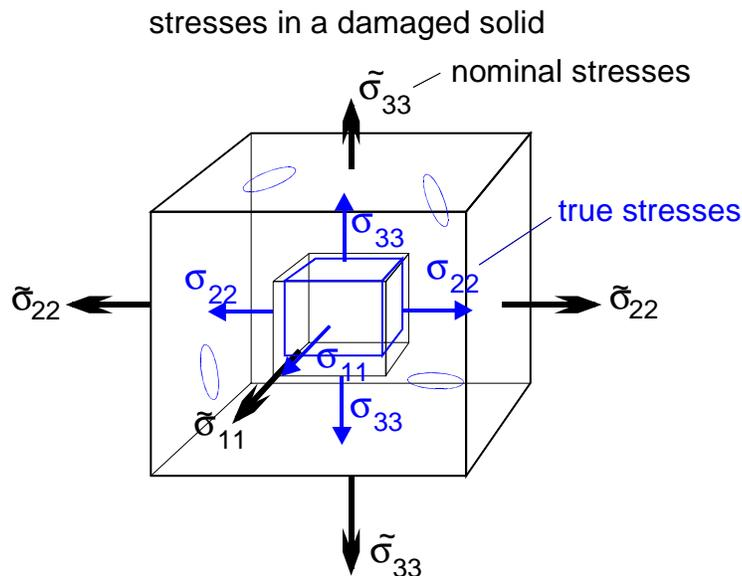
**Figure 12. Definition of true and nominal stresses in a damaging solid.**
