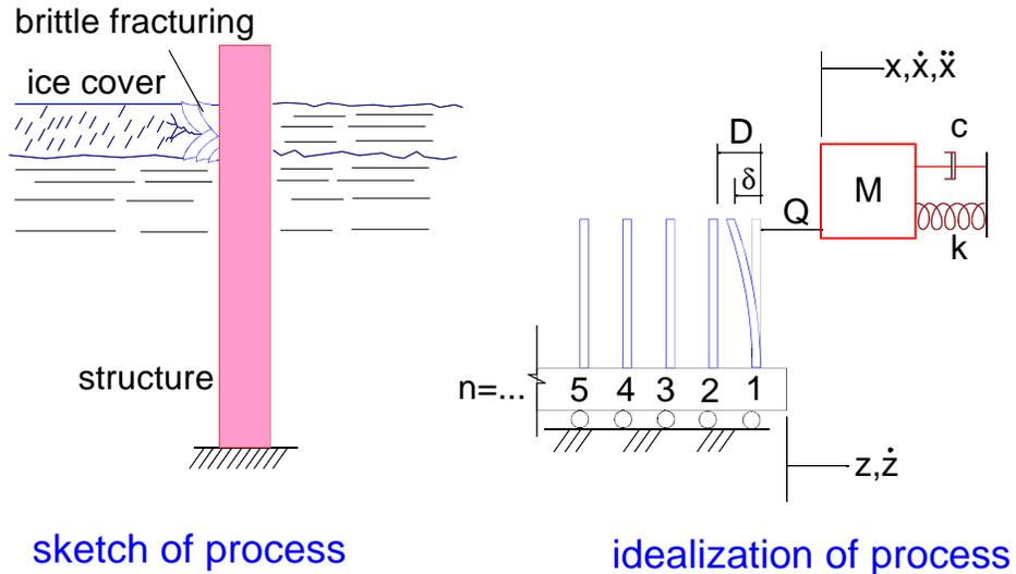
Figure 17. Discrete ice load model (Matlock et. al. 1971).
