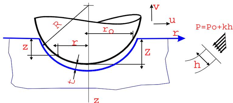
Figure 4. Sphere striking an ice surface. (Kheisin and others, 1975)
