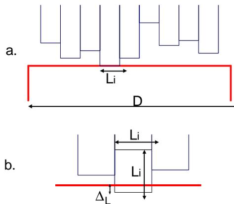
**Figure 13. Non-simultaneous failure model (Ashby et.al., 1986)**
