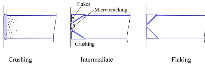
**Figure 9. Failure Modes depending on speed of Indentation (Saeki and Ozaki, 1979)**
