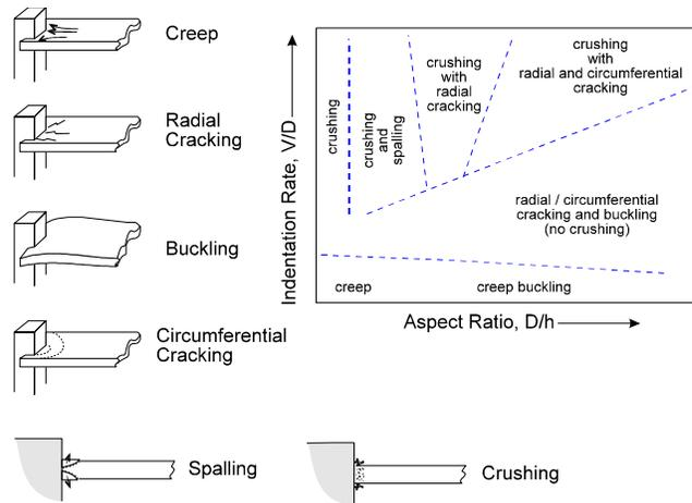
**Figure 11. Failure Mechanisms and Failure Mode Map (Timco, 1986)**
