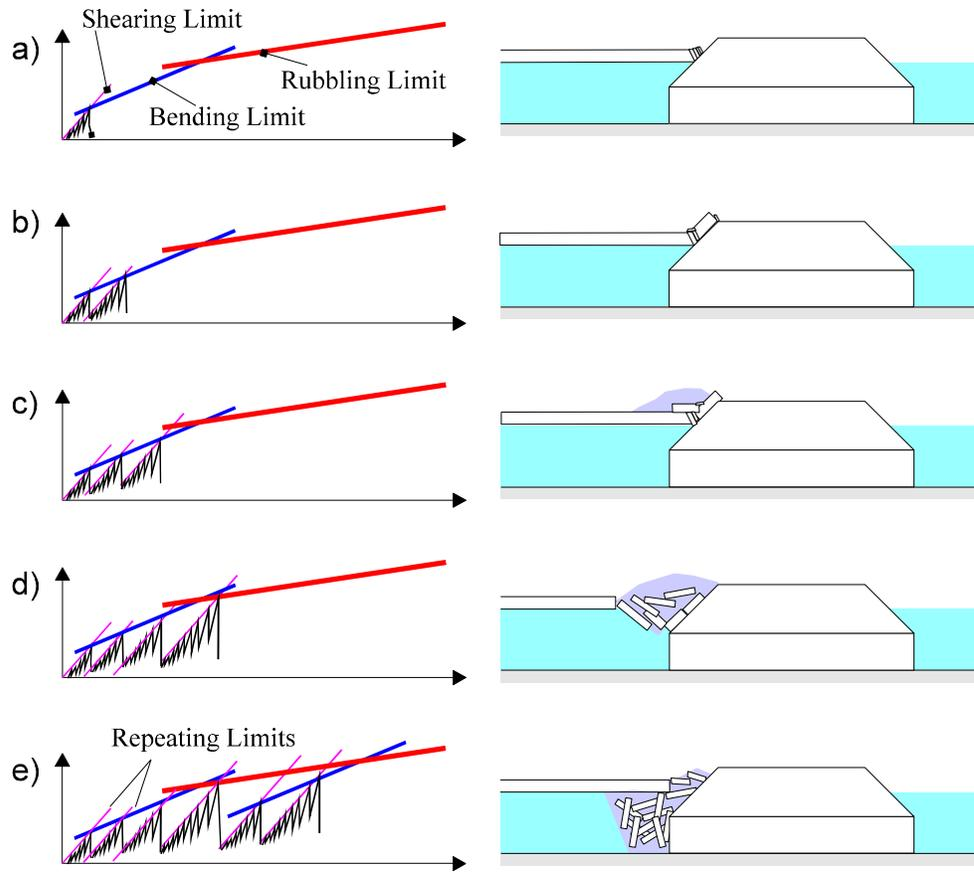
Figure 33. Floe-Structure Interaction showing Hierarchy of Limits
