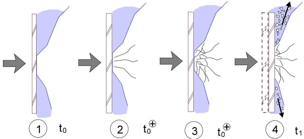
**Figure 28. Pulverization due to a rapid cascade and coalescence of macro cracks**
