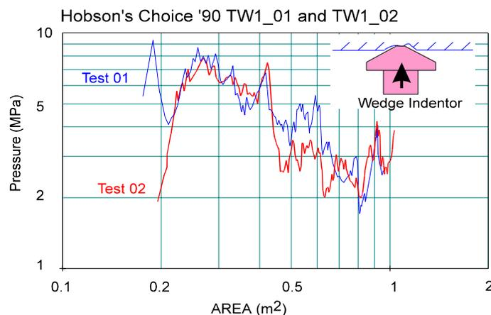
**Figure 40. Two Pressure-Area Records from MSI Tests (Daley, 1994)**
