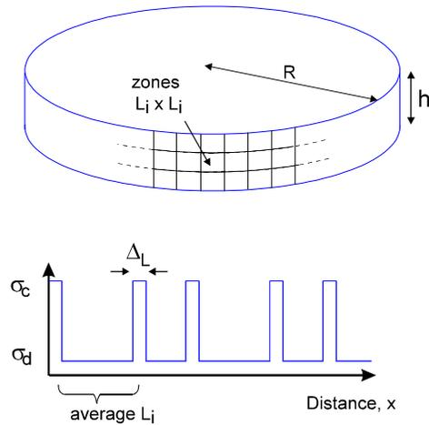
**Figure 14. Multi-zonal stochastic ice edge failure model (Sanderson, 1988)**
