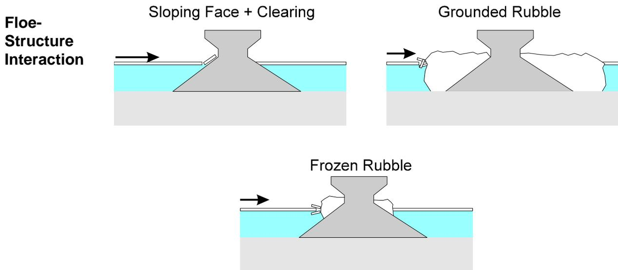
**Figure 32. Floe-Structure Interaction with and without Rubble Formation (Sanderson, 1988)**
