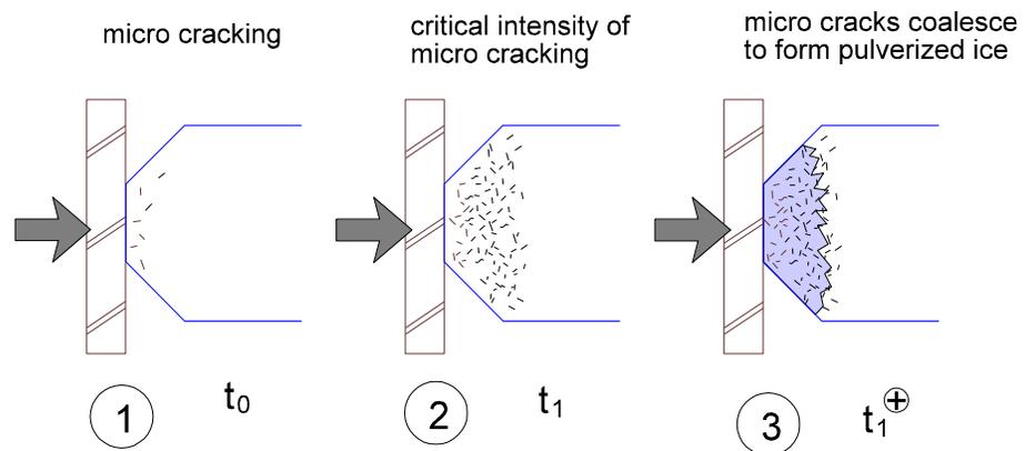
Figure 25. Pulverization due to microcracking.
