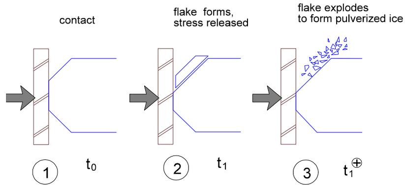
**Figure 26. Pulverization due to flake explosion upon stress release.**
