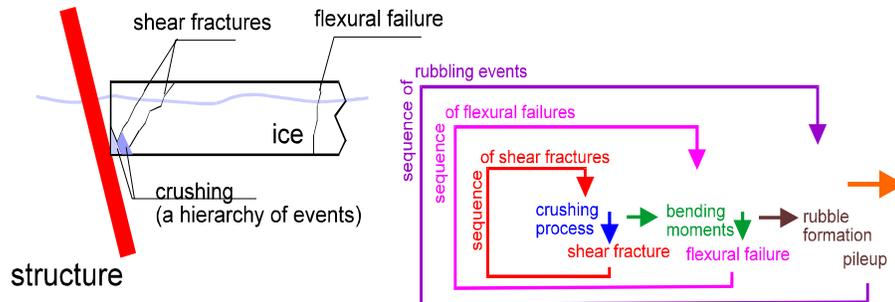
**Figure 3. Nested Hierarchy of Failure Events.**
