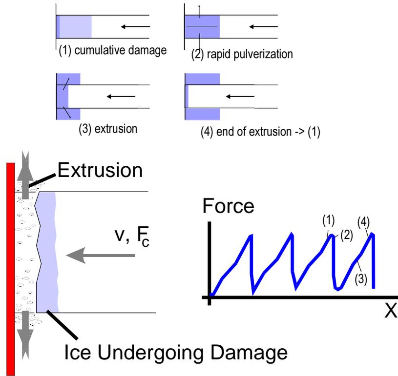
**Figure 7. Finite depth pulverization and extrusion.**
