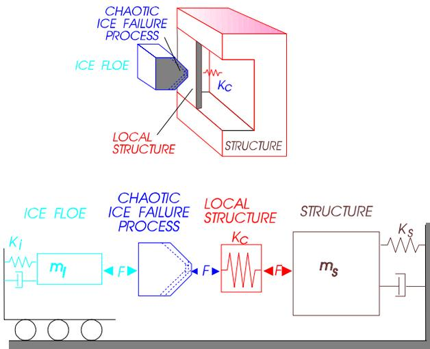
Figure 30. Single Zone Dynamic Ice Load Model (Riska et. al. 1993).
