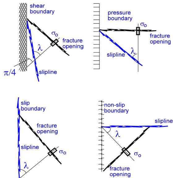
Figure 36. Fracture Mechanics of an Ice Field (Erlingsson, 1988)
