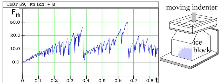
Figure 20. Block crushing tests (test 39, Joensuu and Riska, 1988)
