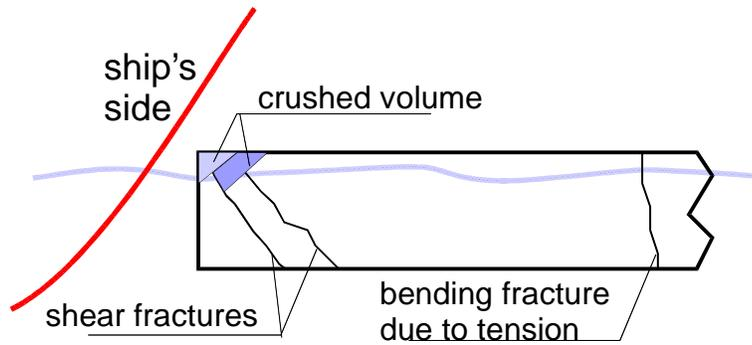
Figure 18. Ice edge failure process on the side of a ship (Varsta and Riska, 1977)
