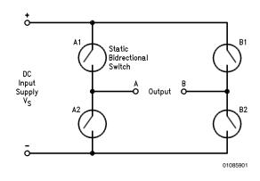
FIGURE 1. Basic H-Bridge Circuit
