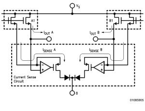
FIGURE 5. The Current Sensing Circuitry of the LMD18200
