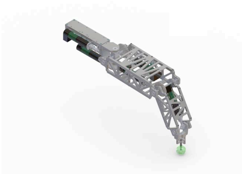
Phase I Hexapod Robot Pre-Production Leg Conceptual design
