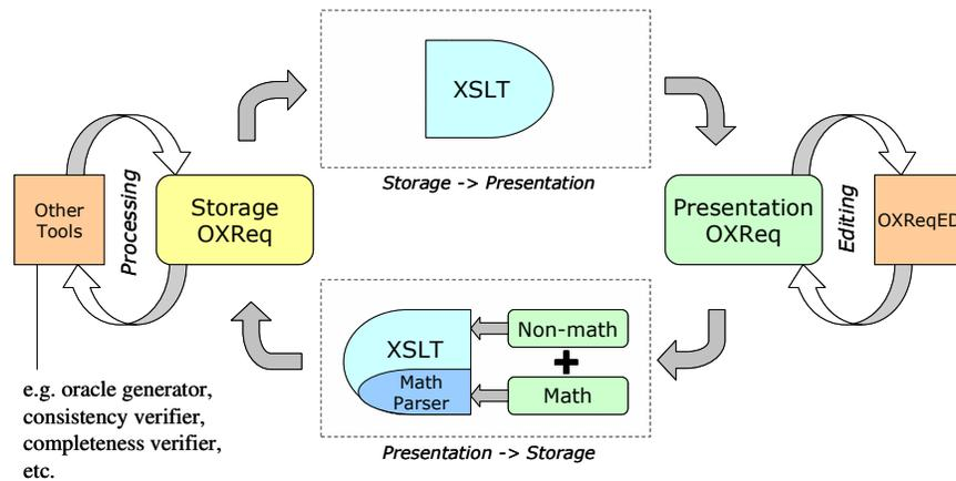
**Figure 2:** The transformation process from storage to presentation OXReq and vice versa
