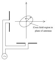
$E_{x} = E_{x_0} \sin(\omega t - kz)$   $E_{y} = E_{y_0} \sin(\omega t - kz + \Delta \phi)$ where  $\Delta \phi$  is phase angle by which  $E_{y}$  leads  $E_{x}$ .
