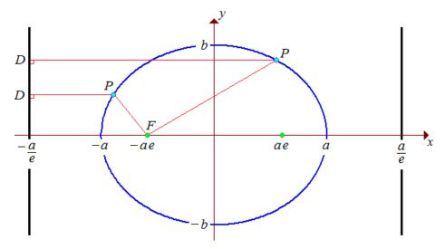
Then the eccentricity *e* is defined as  $e = \frac{PF}{PD}$ The ellipse shown here has an eccentricity e = 0.6.
