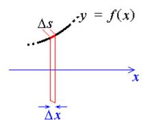
the curved surface area swept out by the element of arc length  $\Delta s$  is approximately the product of the circumference of a circle of radius *y* with the length  $\Delta s$ .
