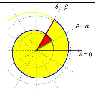
In general, the area bounded by two polar curves  $r = f(\theta)$  and  $r = g(\theta)$  and the radius vectors  $\theta = \alpha$  and  $\theta = \beta$  is
