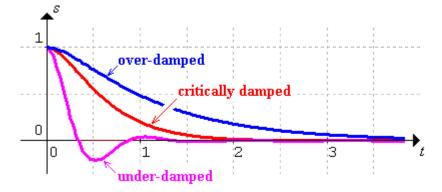
Illustrated here are a critically damped case  $s(t) = (1+3t)e^{-3t}$  (the solution to Example 1.06.1), an over-damped case  $s(t) = \frac{1}{3}(4e^{-t} - e^{-4t})$  and an under-damped case  $s(t) = e^{-3t}(\cos 6t + \frac{1}{2}\sin 6t)$ , all of which share the same initial conditions s(0) = 1 and s'(0) = 0.
