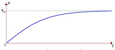
[For a 90 kg person in air,  $b \approx 1 \text{ kg m}^{-1} \rightarrow k \approx 30 \text{ ms}^{-1} \approx 100 \text{ km/h}$ . v(t) is approximately linear at first, but air resistance builds quickly. One accelerates to within 10 km/h of terminal velocity very fast, in just a few seconds.]
