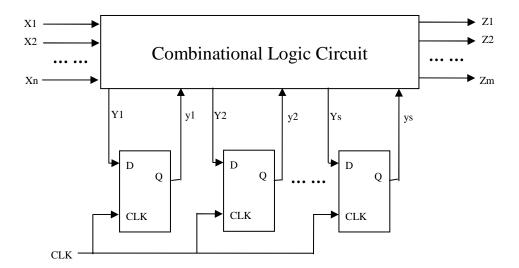
The basic idea: configure all memory elements as units in a shift register (scan) chain.
