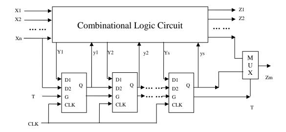
When T=0, D<sub>1</sub> input is the D-input, system operates as usual When T=1, All FFs turn into one long shift register and the combinational logic is bypassed
