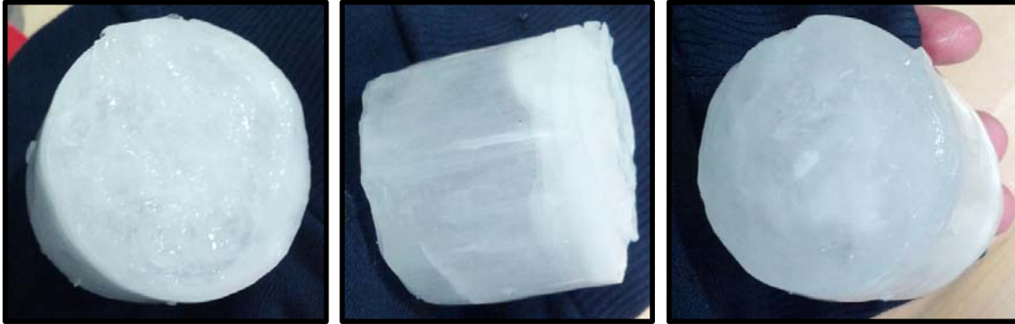
Figure 10. Low speed test remainder portion of ice specimen.
