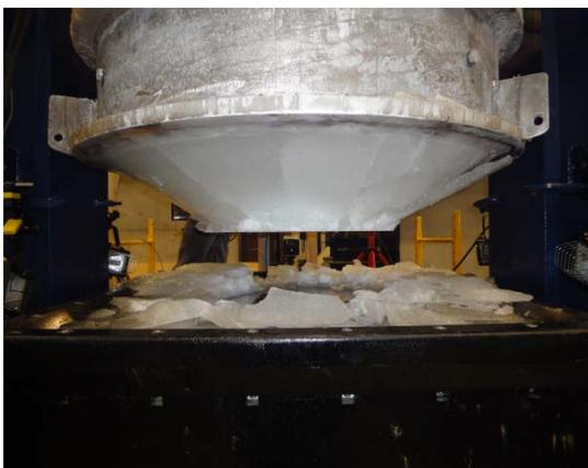
Once all these steps are complete, the ice sample is moved from the cold room and mounted onto the test frame. Different mounting arrangements are used for the two different sized ice samples.
