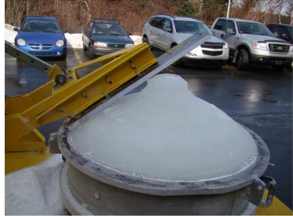
The larger shaping machine works on the same principles as the smaller machine and using this device, the time taken for shaping a large cone is approximately 30 minutes. Once the sample is shaped it's covered using an insulating jacket until it is further used for a test. In this way both small and large ice cone samples are prepared.
