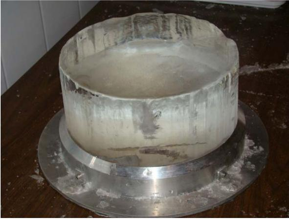
**Figure 2 Shaping of Small Cone Sample**
