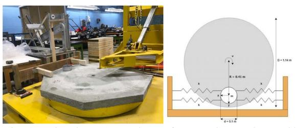
Figure 1: Experimental set-up: a) Ice sample support frame next to the octagonal concrete slab on the turntable; b) top view showing the dimensions and degrees of freedom.
