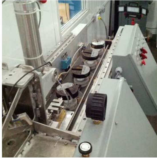
Figure 7 Samples with 2.25 kg weights, after 24 hours of loading, ready for testing. Weights were removed immediately prior to the start of the tests.
