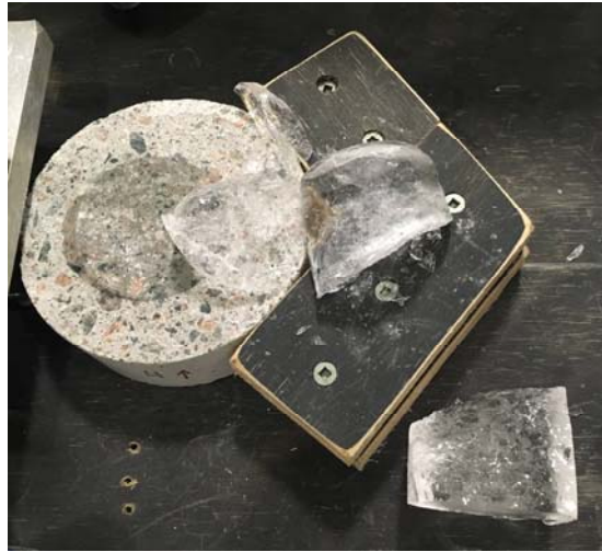
Figure 9 Example of catastrophic cohesive failure during a preliminary test.
