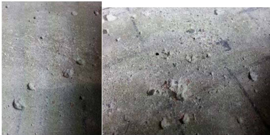
Figure 9 Concrete abrasion on the high performance concrete sample (left) and low performance concrete sample (right) over a test sequence. The location is at the starting point of the test runs as shown with the cross in Figure 3. The loading on the high performance concrete sample is much higher than for the low performance concrete sample. The grid lines (20 mm distance) provide reference.
