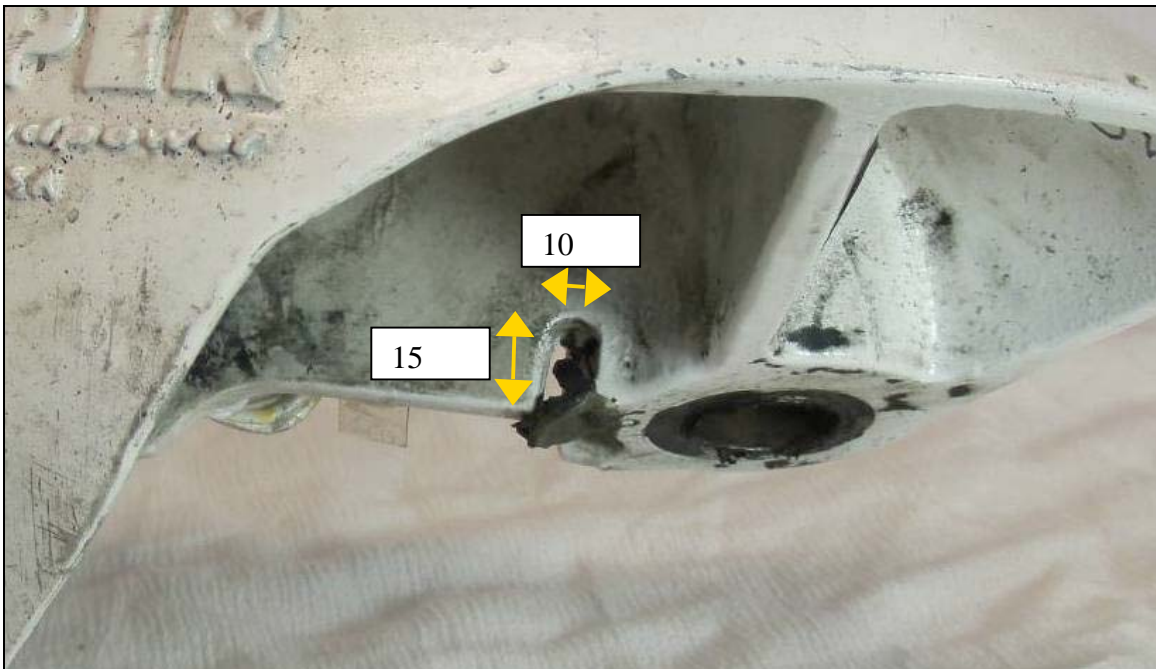
Figure 4.8 – Close up of the notch of an intact WH100 nacelle
