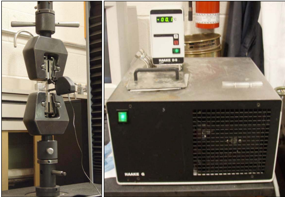
Figure 4.13 –Tensile test being performed (left) and constant temperature bath (right)
