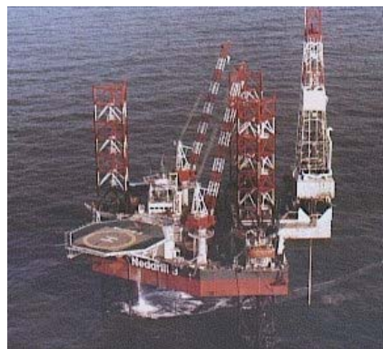
Slide 3 : Cantilevered drilling rig: Self-elevating (jack-up) exploration drilling platform.
