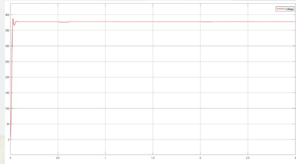
Fig. 27: Output voltage of the second DC-DC converter stage.
