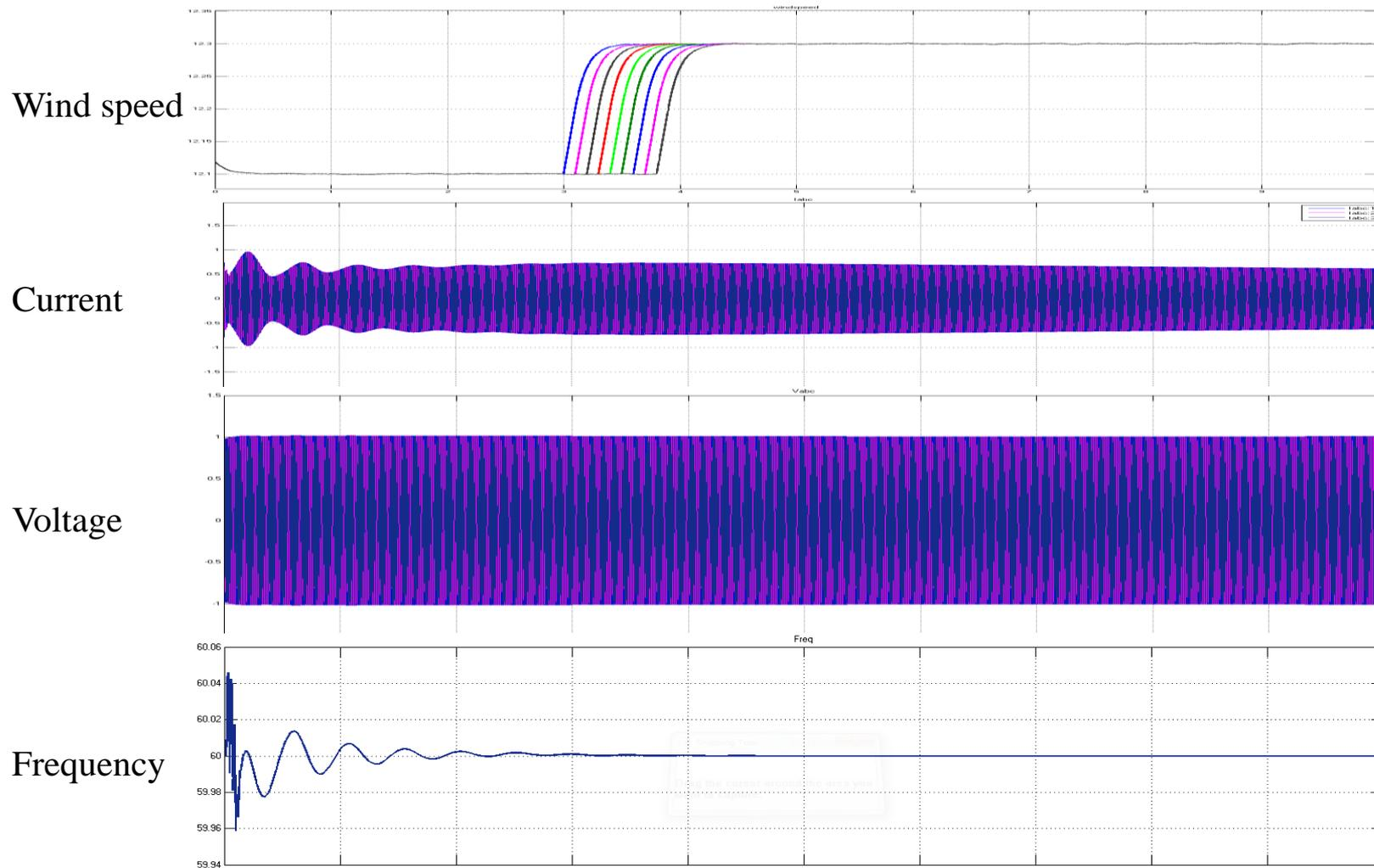
(3) The wind farm trips due to a fault and then reconnects to the grid.
