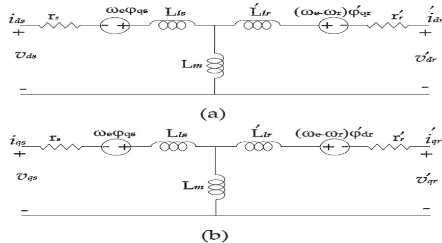
Equivalent circuit in synchronously rotating reference frame: (a) d-axis; (b) q-axis
