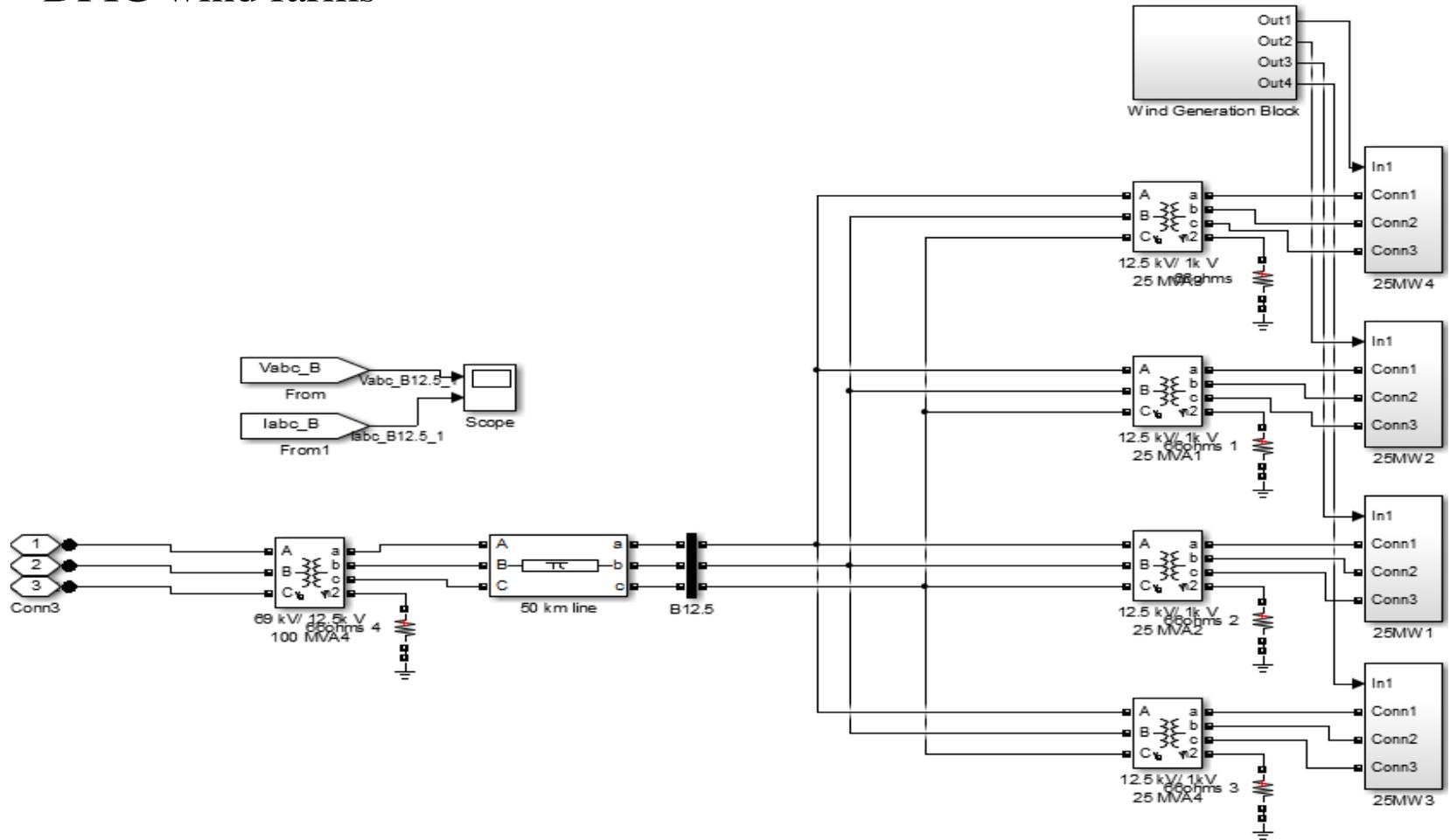
Modeling of each 100 MW capacity wind farm made of four 25 MW wind farms
