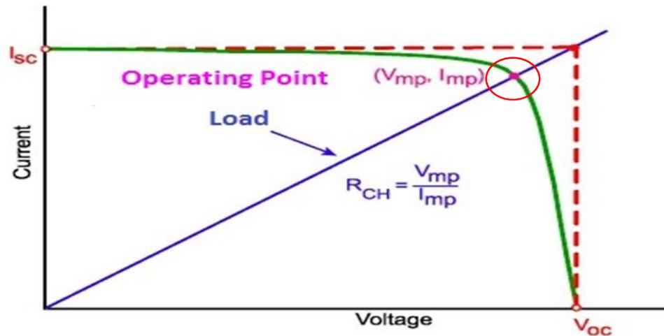
Load matching of a PV panel with a given insolation; Match power using MPPT
