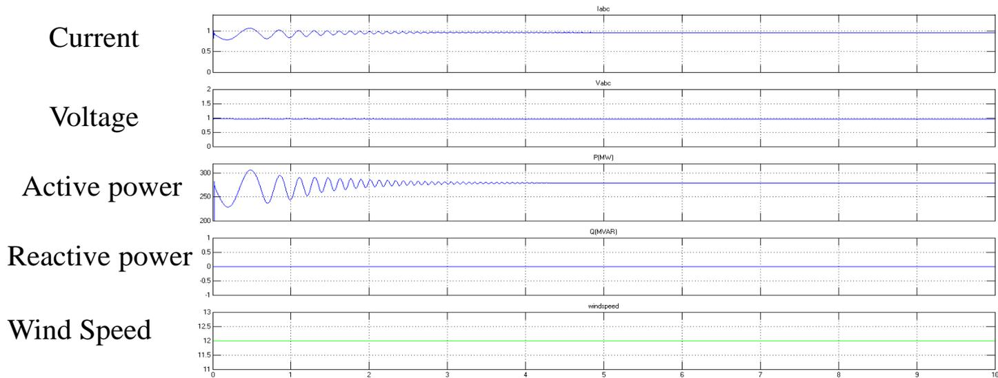
Current, voltage, P and Q scopes at constant wind speed
