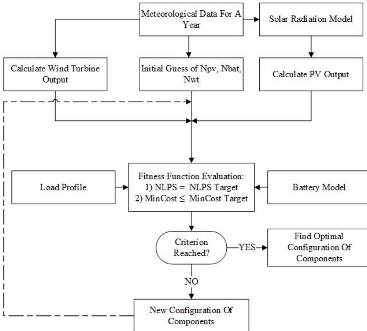
Algorithm for optimal sizing the system
