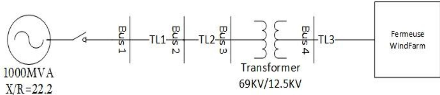
Fermeuse wind farm grid connection single line diagram
