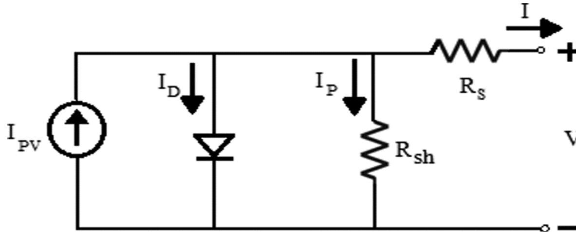
Equivalent circuit of a PV module
