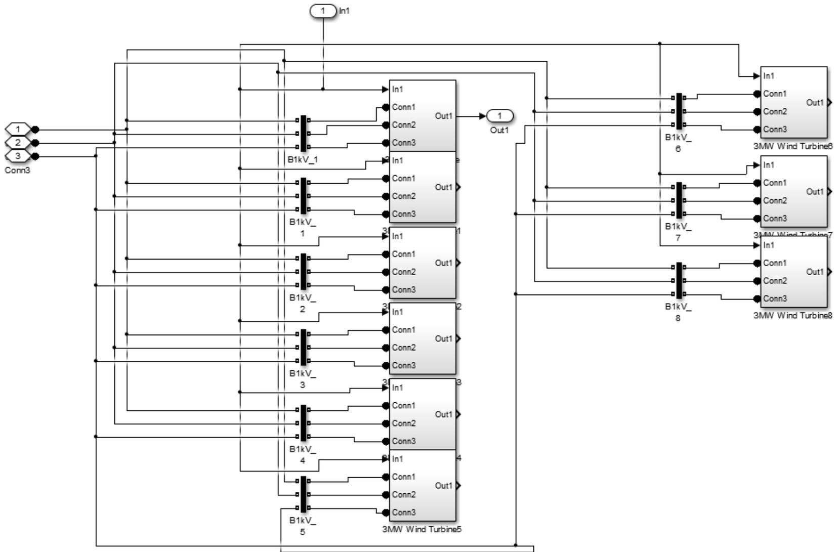
Details of a 25MW wind farm model in Simulink (9\*3MW)
