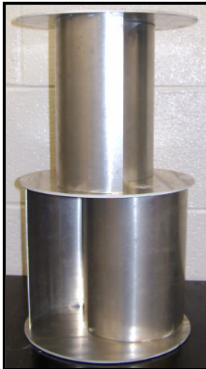
Fig: Two-Stage Savonius
