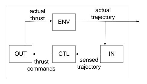
The set of trajectories possible is  $S = \{x \mid x(\textit{ENV} \circ \textit{OUT} \circ \textit{CTL} \circ \textit{IN})x\}$ If the requirement is specified as a set of allowable trajectories, *R*, then we must design the system so that  $S \subseteq R$
