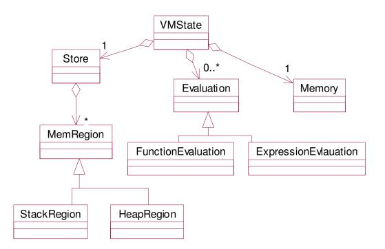
Some of the Classes within the VirtualMachine package.  $C \longrightarrow P$  means C *is a specialization* of P. I.e. C *inherits from* P.
