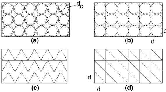
Fig. 4. Some possible packing arrangements: (a) Circumscribed polygons; (b) square ducts; (c) equilateral triangle; and (d) isosceles right triangle.
