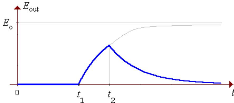
The capacitor charges from 0 at time \$t\_1\$ then discharges from time \$t\_2\$ onwards.
