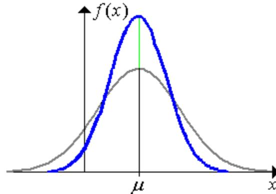
Because there is no closed algebraic form for the *c.d.f.*  $F(x)$ , the values are tabulated for one special choice of mean and variance:  $\mu = 0, \sigma^2 = 1$ .
