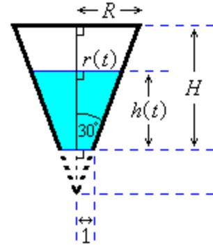
The rate at which the volume  $V(t)$  of liquid in the tank changes due to liquid draining at discharge speed  $v(t)$  through a hole of area  $A$  is given by the differential equation
