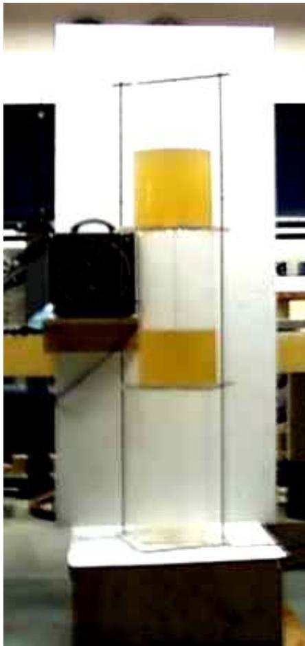
Figure A1. Ensure that the above apparatus is level, so that the tank walls are vertical.
