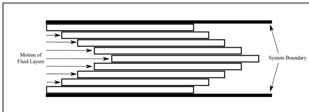
Solvent in laminar flow moves as sliding layers with different velocities
