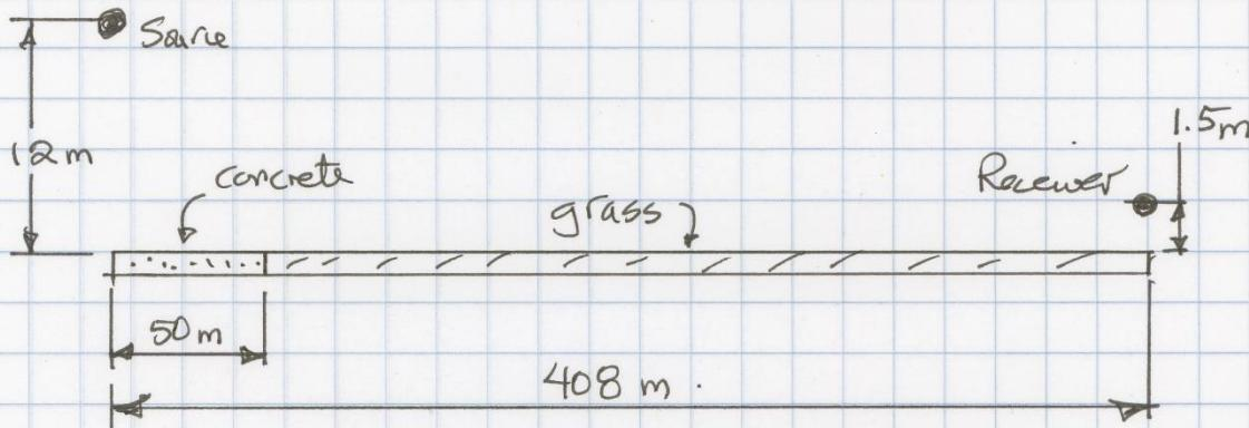
$$\text{Source zone} = 30 \text{ hs} = 30(12 \text{ m}) = 360 \text{ m.}$$
