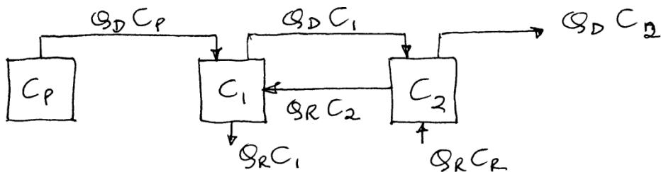
mass balance equation  $Q_D C_P + Q_R C_2 = Q_D C_1 + Q_R C_1$
