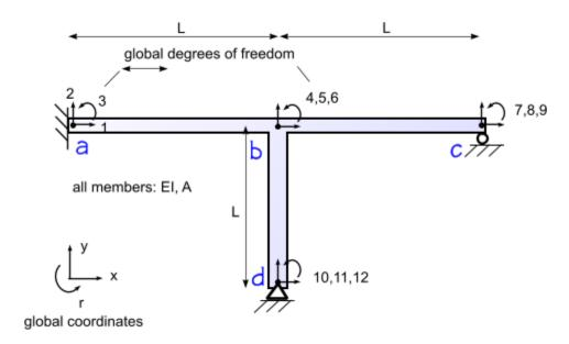
D of F 4 is the x movement at node 'b'.  $k_{4,4}$  is the sum of the axial terms from beam a-b and b-c plus the shear term from beam b-d.  $k_{10,10}$  is the shear term from beam b-d.
