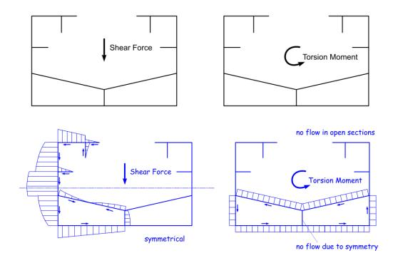
b) A cross section of a box girder is shown below. A vertical shear force of 2 MN is applied. Solve the shear flow, plot it and then also show the shear stress values (9).
