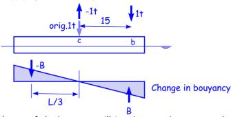
B the change of the bouyancy will just be more buoyancy under one end and less under the other end, with no change in buoyancy at midships. Each half of the buoyancy change is termed B with a center of effect at 2/3 of the half length. The magnitude of B must enough to create a moment to exactly counteract the moment caused by the shifted weight:
