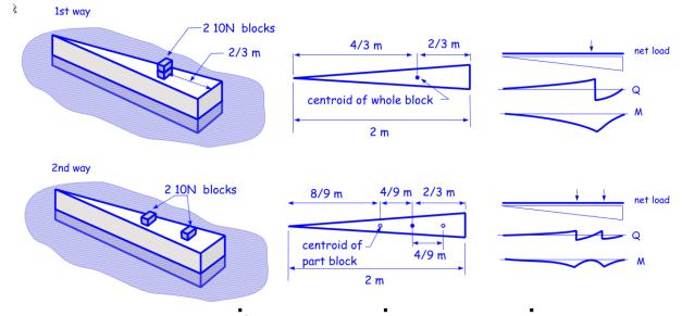
the two small blocks must have their combined center of gravity at the same point as the triangular block (so no moment occurs to cause trim). The two blocks can be moved equally left and right. Likely mimimum bending will occur when blocks are over the centroids of the left and right parts of the triangular block. So second way causes less bending.
