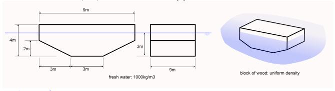
Submerged area = 21 m2 Submerged volume = 189 m3 Mass of floating body is 189,000 kg
