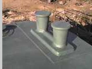
Double post bitt. A single post item similar to this would be a bollard. It is easier to secure and remove a rope on a double post bitt.
