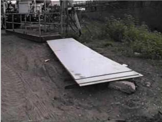
A stack of plates that will be used for side shell replacement, frames, brackets, etc.... These plates have been sandblasted and coated to reduce corrosion inside the vessel once they are installed.
