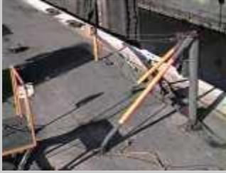
Here is a **davit**, or a **cargo hose boom**. This one design of several different types of devices designed to assist in lifting heavy items. The **King Post** or **Sampson Post** or **Stanchion** is the vertical pipe on the right side of the picture. The **boom (spar)** extends to the left, and is supported by a boom rest near the tip, and the **boom socket (step)** at the base of the **king post**.
