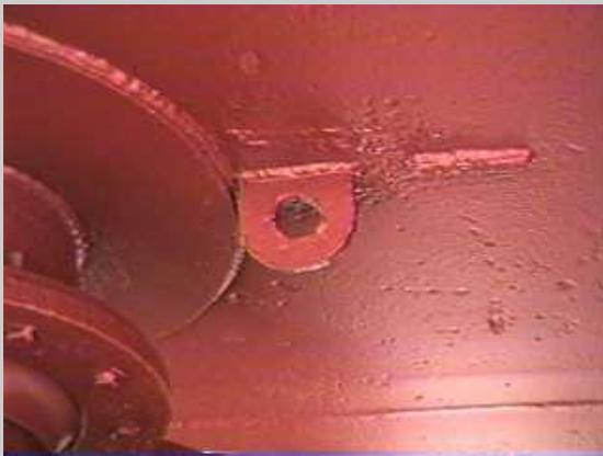
This pad eye is just forward of the rudder, and would be used to hold a chain fall when the crew are working on the propeller. In this picture, the vessel is on dry-dock, and we are looking up at the bottom of the hull.
