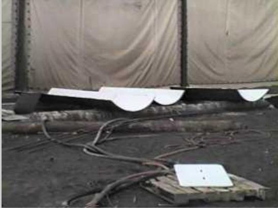
Knuckle plates. These plates have been shaped to the exact radius needed for the vessel. They have been sandblasted and coated on the inside to stop corrosion inside the vessel.
