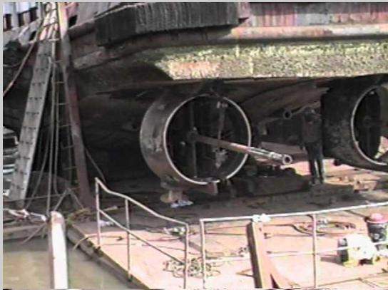
Kort nozzles are engineered to improve the flow around the propellers. They are similar in some ways to an airplane propeller. The propeller shaft on this vessel is being 'pulled'. Propulsion systems on vessels are inspected and worn parts are replaced at each drydock opportunity.
