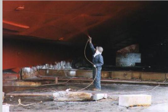
ainter applying a coating to a vessel hull.
