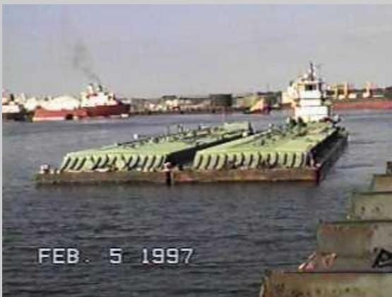
These 2 **tank barges** are loaded with petrochemicals in the Houston, Texas, USA ship channel. The boat that is pushing them is called a **tow boat**, because it pushes a 'tow of barges'.
