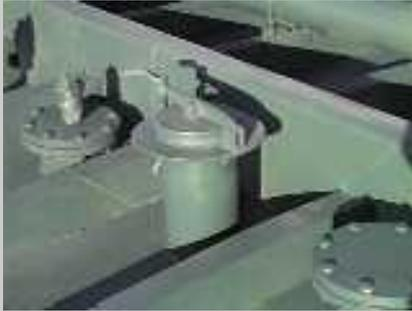
Ullage hatch used for gauging the ullage or innage of a cargo.
