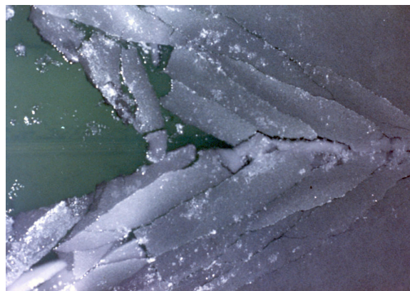
Figure 10.9 Bow-print showing the broken ice pattern for a ship model
