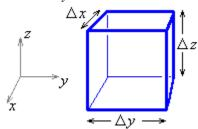
The front face is at  $(x + \Delta x)$  and the back face is at (x).
