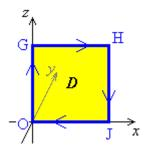
Because of the right-hand rule, the positive orientation around the square is OGHJ (the *y* axis is directed into the page).
