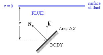
The pressure at any depth z is the weight of fluid per unit area from the column of fluid above that area. Therefore
