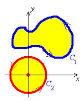
Green's theorem is valid for curve  $C_1$  but not for curve  $C_2$ . There is a singularity at the origin, which curve  $C_2$  encloses.
