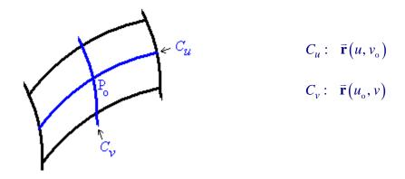
If, instead, u is held constant at  $u_0$  and v is allowed to vary, we obtain a different slice containing  $P_0$ , the curve  $C_v$ :  $\bar{\mathbf{r}}(u_0, v)$ .
