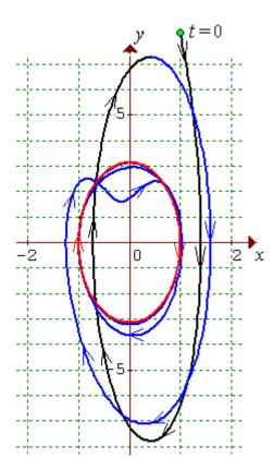
This ellipse must therefore be the limit cycle for the system.
