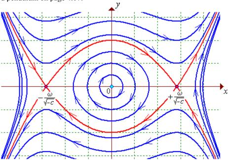
The orbits passing through the saddle points separates closed orbits from open orbits and is called the **separatrix**.
