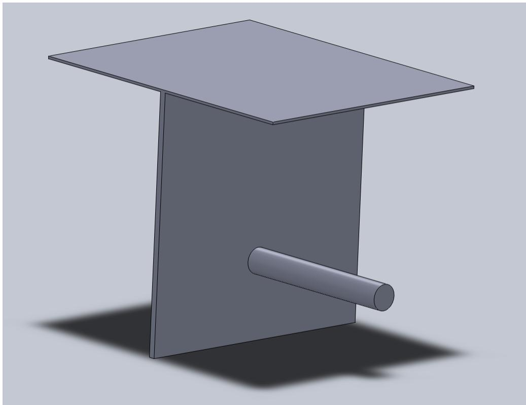
The horizontal force is pressure at center of the circle times the profile area
