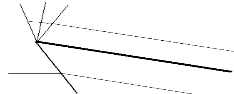
The expansion wave plot gives  $v=55$  for upstream Mach Number  $M=3$ . Adding attack angle 25 to this gives  $v=80$  on top of the foil. The plot gives  $M=5.5$  for top of foil. Substitution into the isentropic pressure ratio equation gives:
