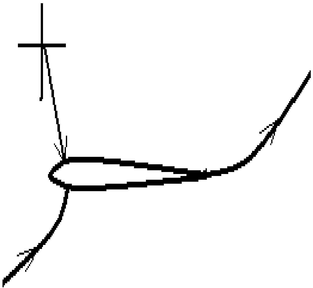
Explain how you would calculate lift on a Joukowsky foil from calculated pressure. What is the theoretical lift on the foil?
