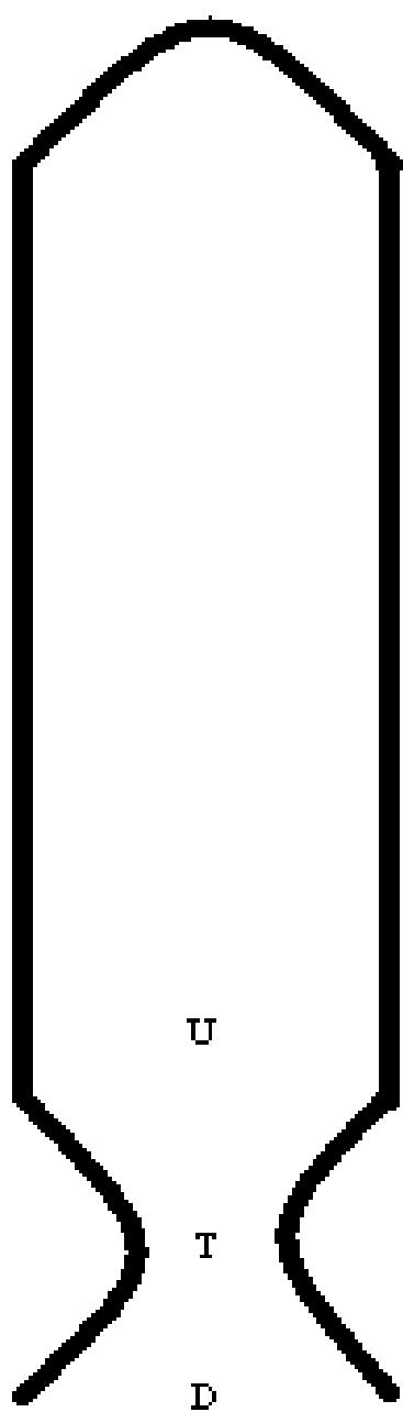
Explain how you would calculate the pressure and flow velocity changes which occur when a high speed flow moves down a pipe. Identify the important equations. [15]
