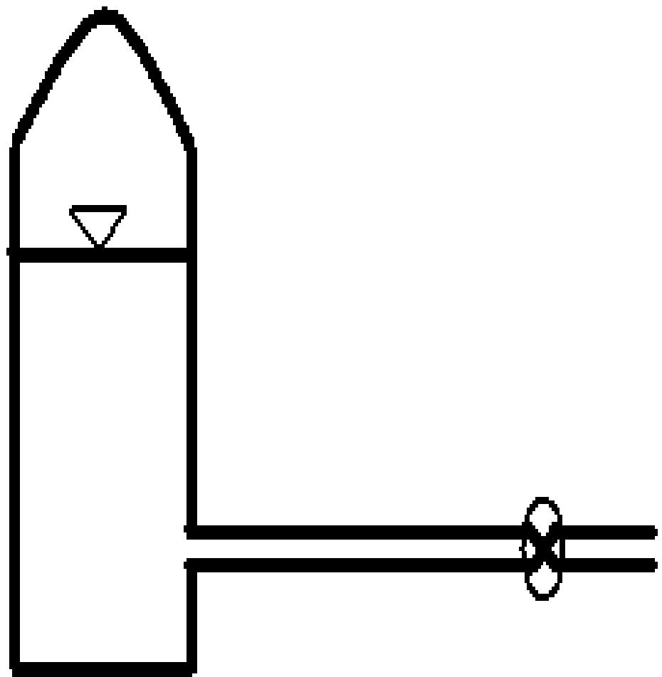
Consider a small deadend pipe attached to a large pipe with a valve at its downstream end and a large pressurized tank at its upstream end. Using algebraic waterhammer concepts, explain how you would calculate pressure and flow velocity in the deadend pipe following a sudden valve closure in the large pipe. Sketch the PU plot for the deadend pipe. [15] Identify the important equations.
