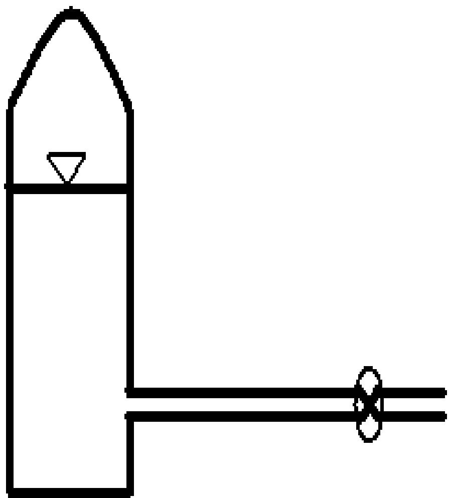
Consider a small deadend pipe attached to a large pipe with a valve at its downstream end and a large pressurized tank at its upstream end. Using the method of characteristics, explain how you would calculate the pressure and flow velocity at 3 points in the deadend pipe following a sudden valve closure in the large pipe. Do surge wave case only. Use waterhammer analysis if you cannot remember method of characteristics. Identify the important equations. [15]
