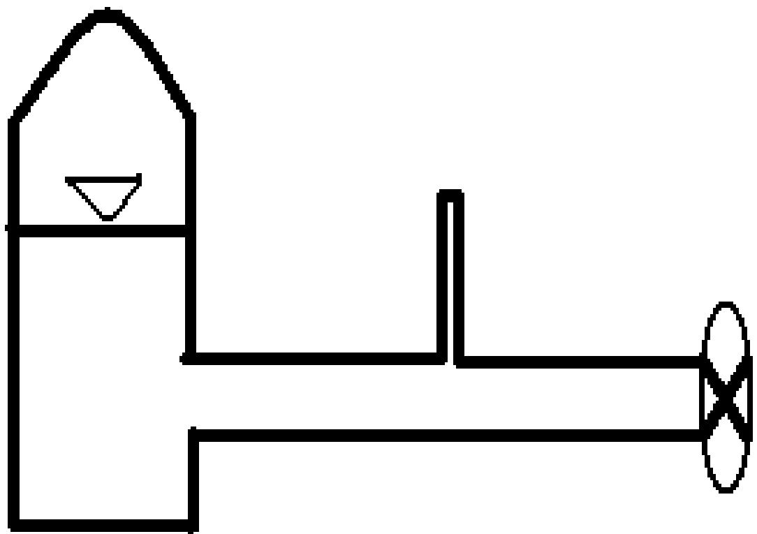
Let A B C indicate present pressure and flow velocity at 3 points along the deadend pipe: A is at the entrance to the deadend pipe, B is in the middle of the deadend pipe and C is at the deadend. Let I J K indicate pressure and flow velocity a step forward in time at the corresponding points. At the entrance the pressure is the surge pressure  $P_s$ . At the deadend the flow velocity is zero.
