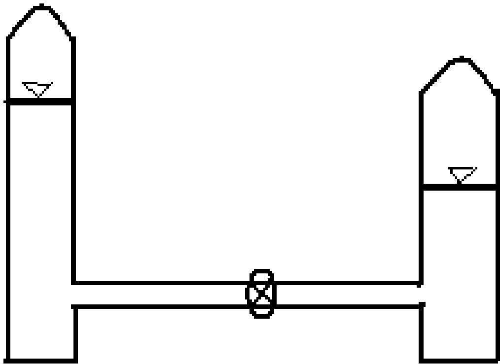
When the valve is suddenly closed, it creates a flow imbalance. A low pressure or suction wave is created which propagates down the pipe. As it does so, it brings the fluid to rest. The pipe has low pressure all along its length.
