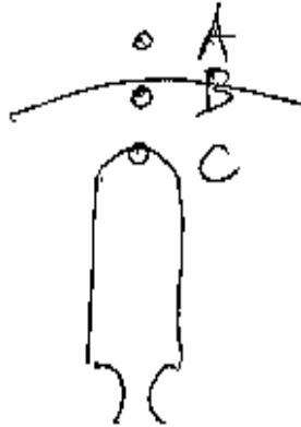
For rocket moving at low Subsonic speed  $\Rightarrow$  stagnation point pressure
