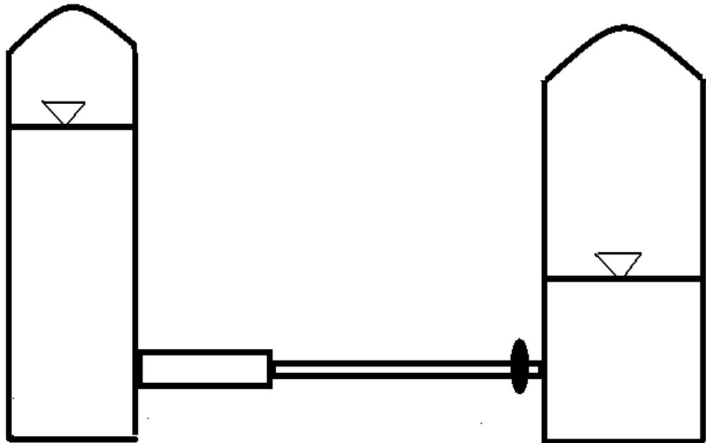
The downstream pipe is twice as long as the upstream pipe, and it has a wave speed that is half that of the upstream pipe. This means that its transit time is 4 times that of the upstream pipe. This implies it must be divided into 4 reaches. The sketch below shows a typical reach point:
