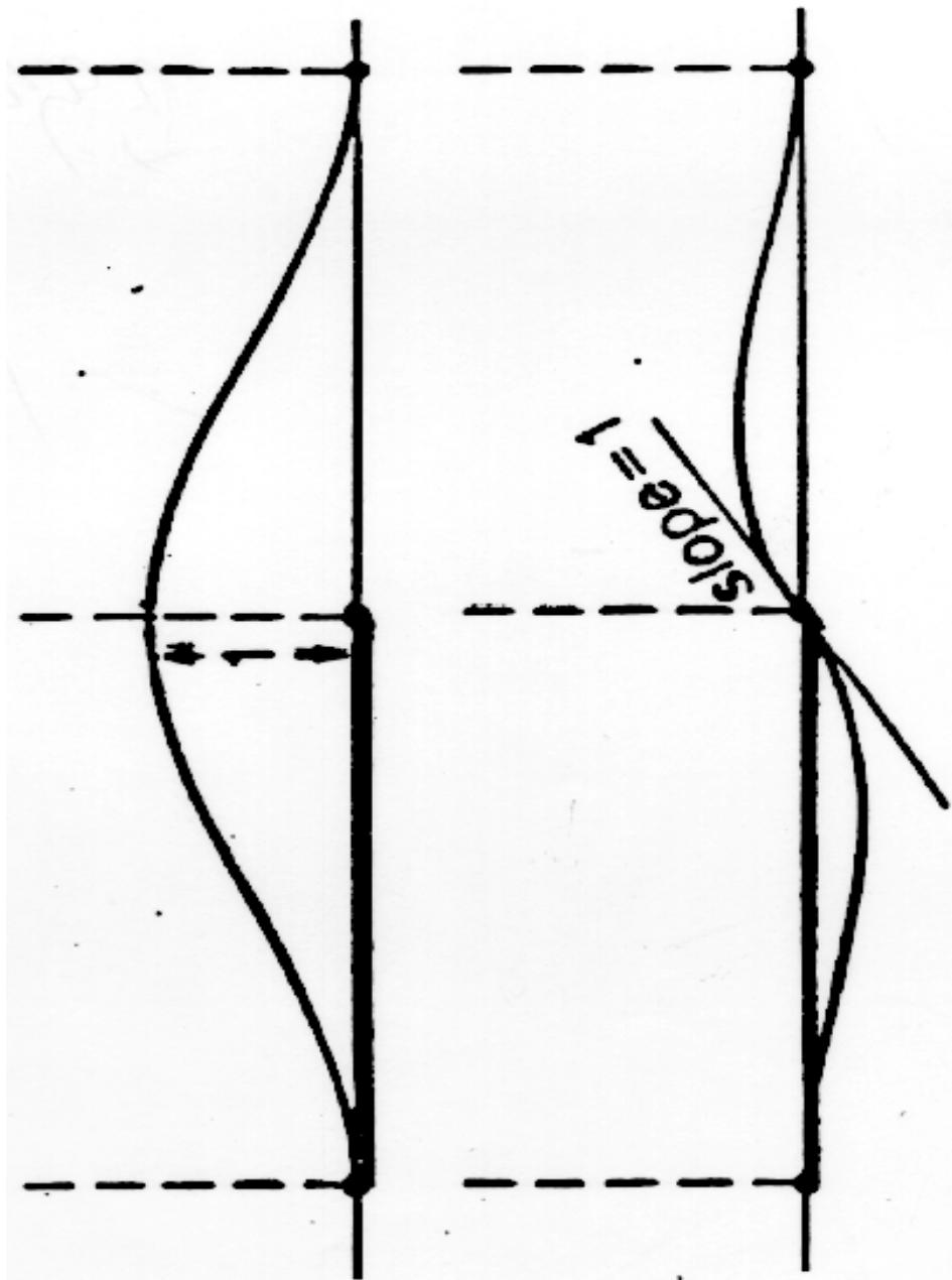
Substitution of the assumed form for  $\mathbf{Y}$  into the governing equation gives a residual  $\mathbf{R}$ . In a Galerkin analysis, weighted averages of this residual along the pipe are set to zero:
