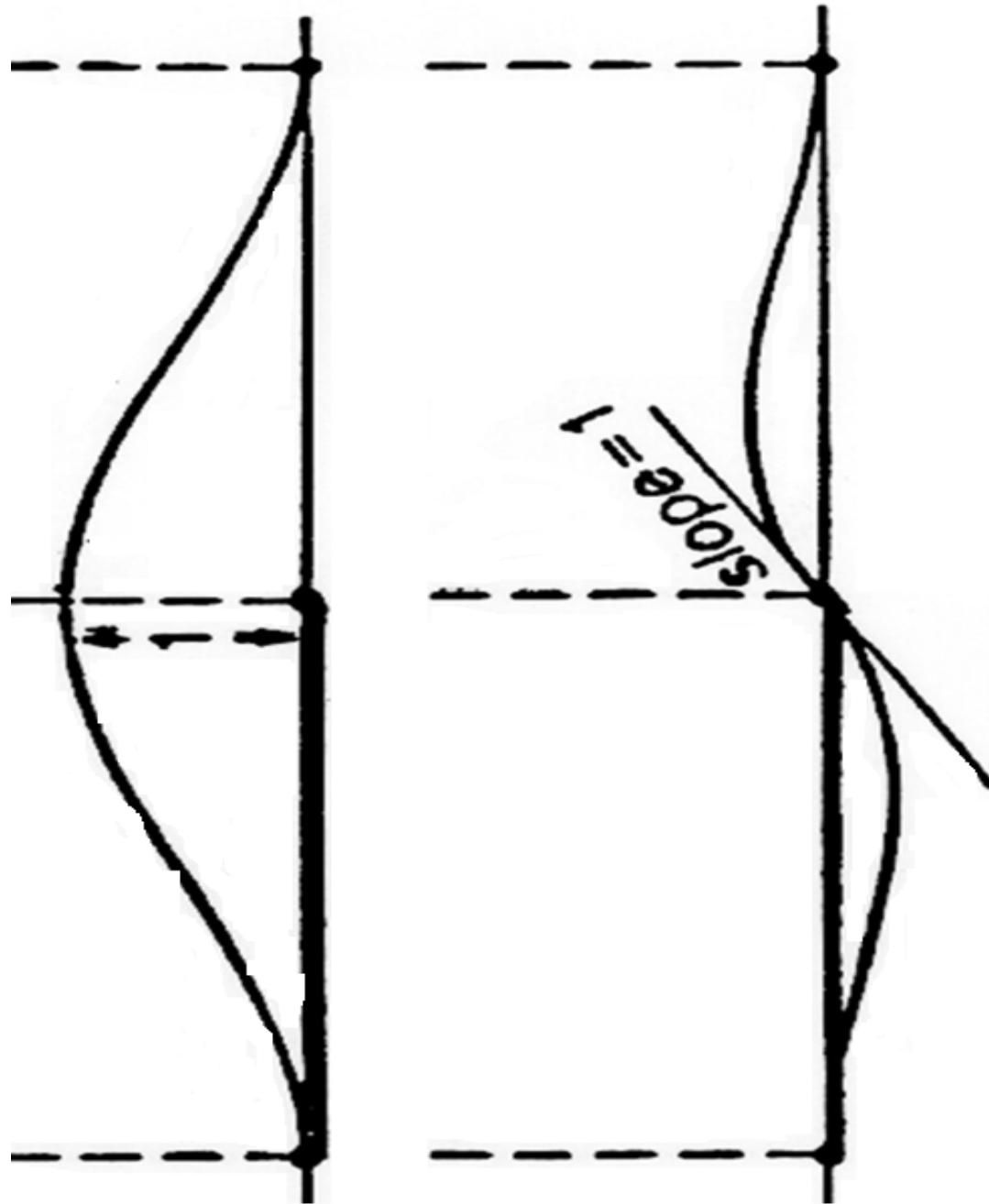
Substitution of the assumed form for  $\mathbf{Y}$  into the governing equation gives a residual. In a Galerkin analysis, weighted averages of this residual along the beam are set to zero. After some manipulation, one gets
