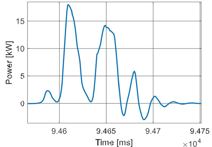
*Switching Loss During Cut-Off at H-Bridge Silicon Carbide Switch*
