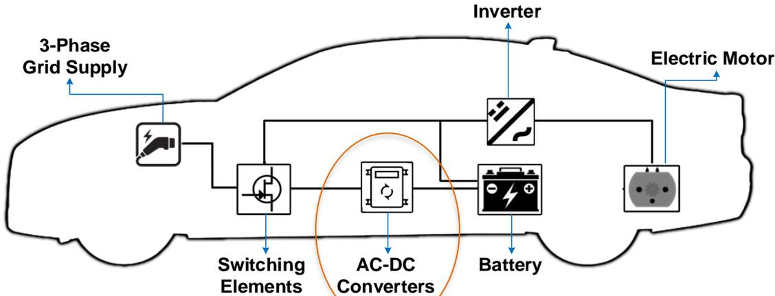
Figure: Conventional AC-DC On-Board Charger Design
