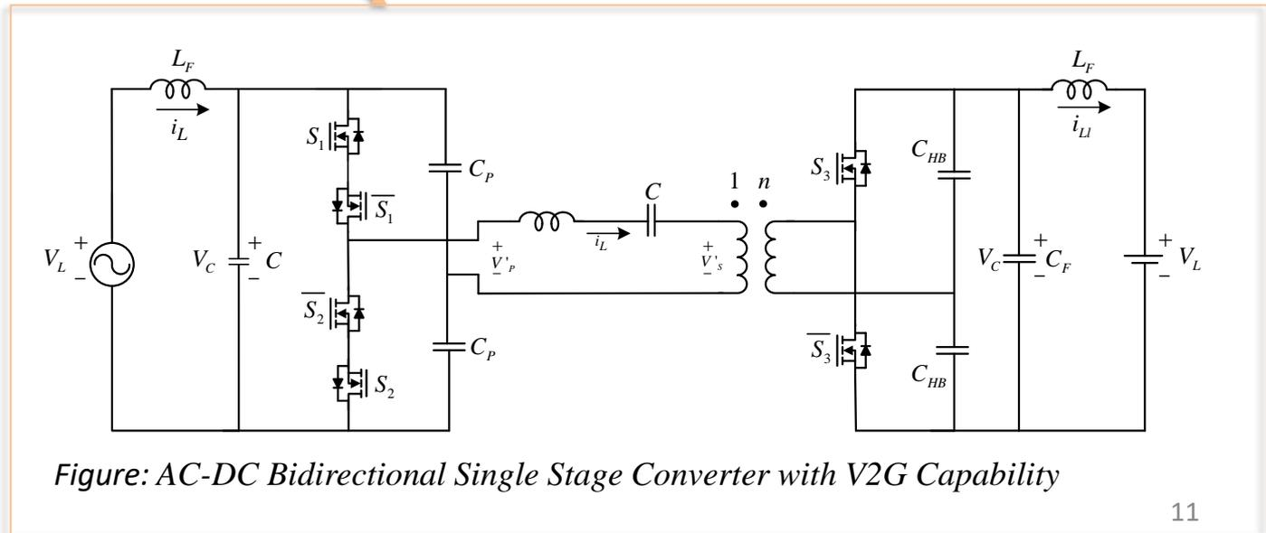
Figure: AC-DC Bidirectional Single Stage Converter with V2G Capability
