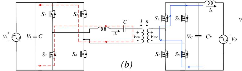
Figure b. CC Charging Mode of Operation
