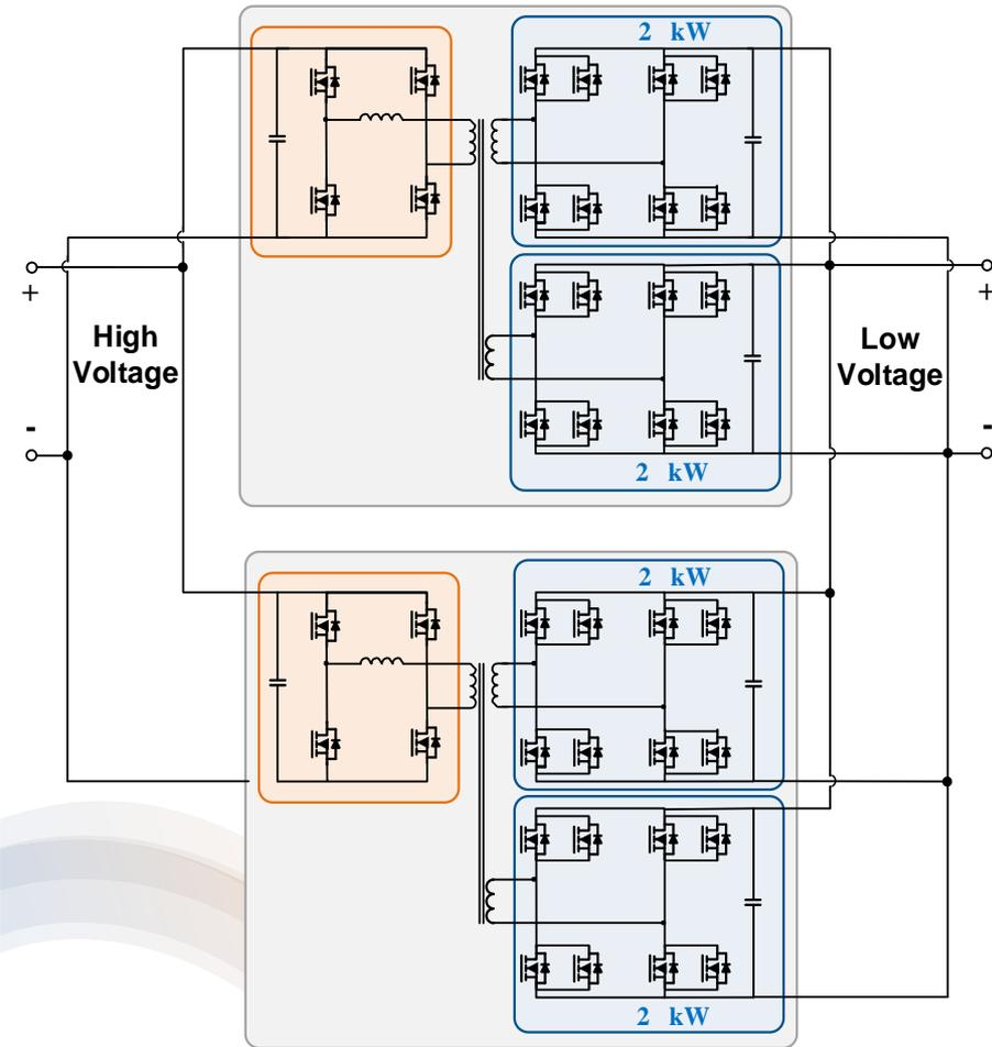
*Figure. Connection-2 for the 4 kW Converter*
