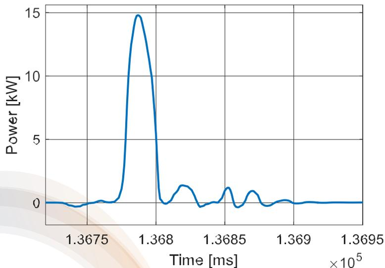
*Switching Loss During Conduction at H-Bridge Silicon Carbide Switches*
