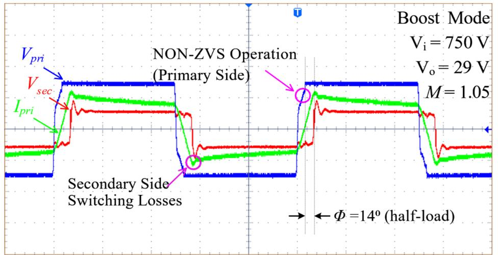
*Waveforms of the Converter Operation for Boost Mode*
