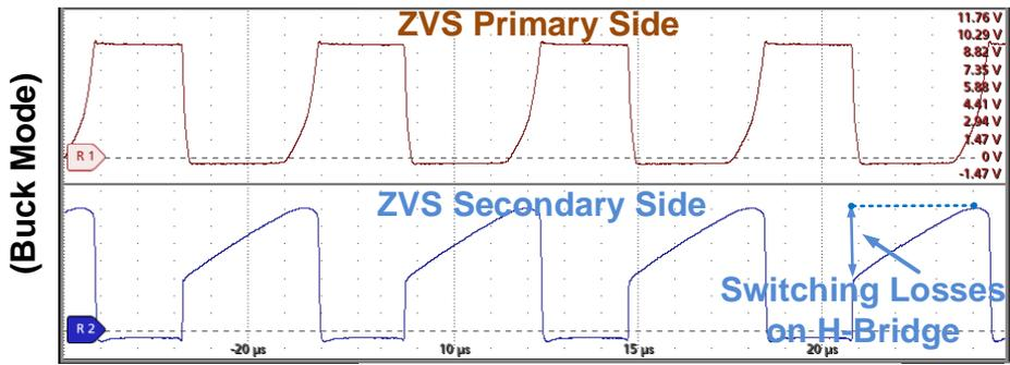
Figure. Waveforms for Buck Mode
