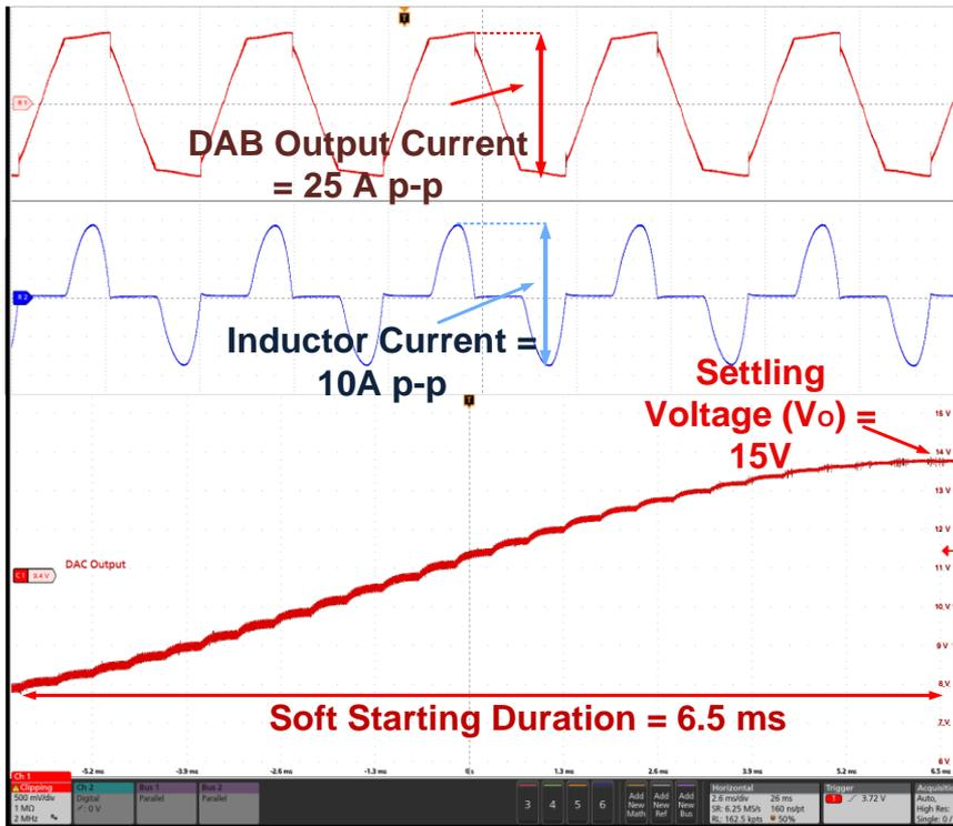
Figure. Converter voltage and the energy transfer inductor current
