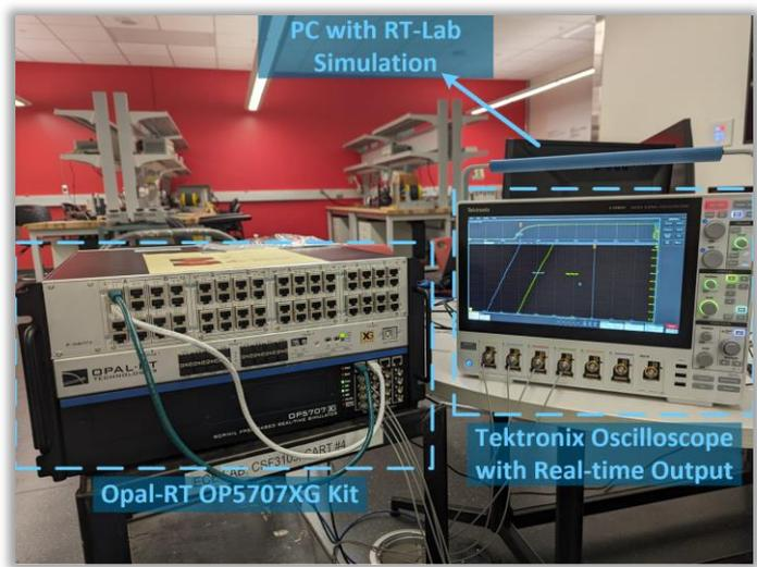
Figure: Hardware Validation Lab Setup
