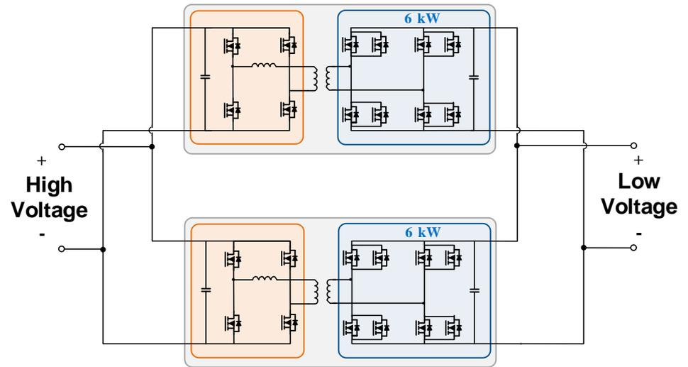
*Figure. Connection for the 11.5 kW Converter*
