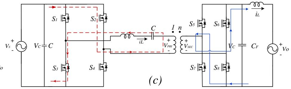
Figure c. CV Charging Mode of Operation
