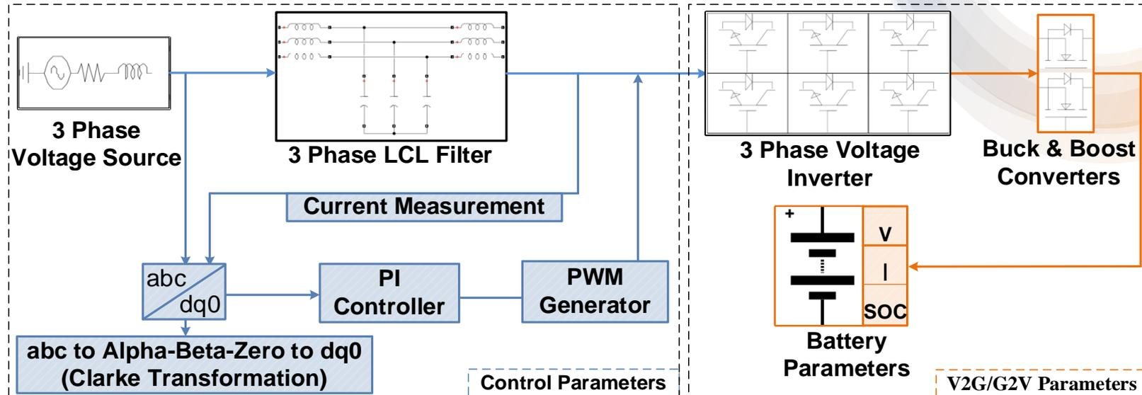
Figure. Block Chart for Control Methodology
