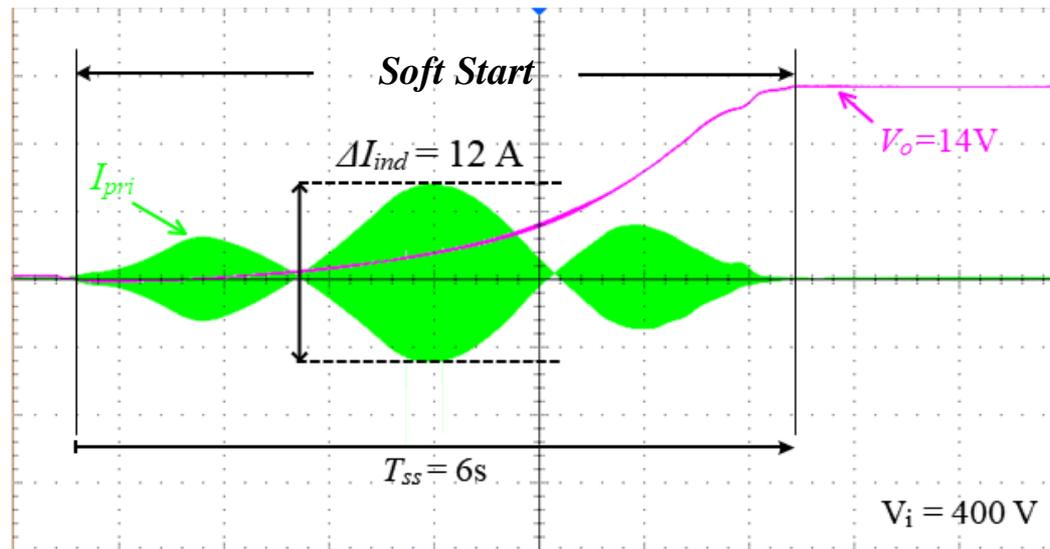
*Primary Current of the Transformer and Converter Output Voltage During Soft Start*
