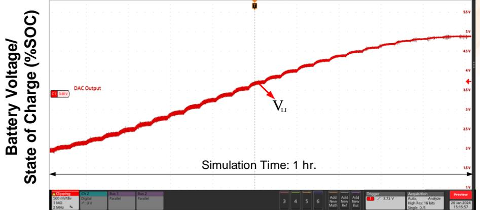
Figure. Real-Time G2V SOC% Outputs
