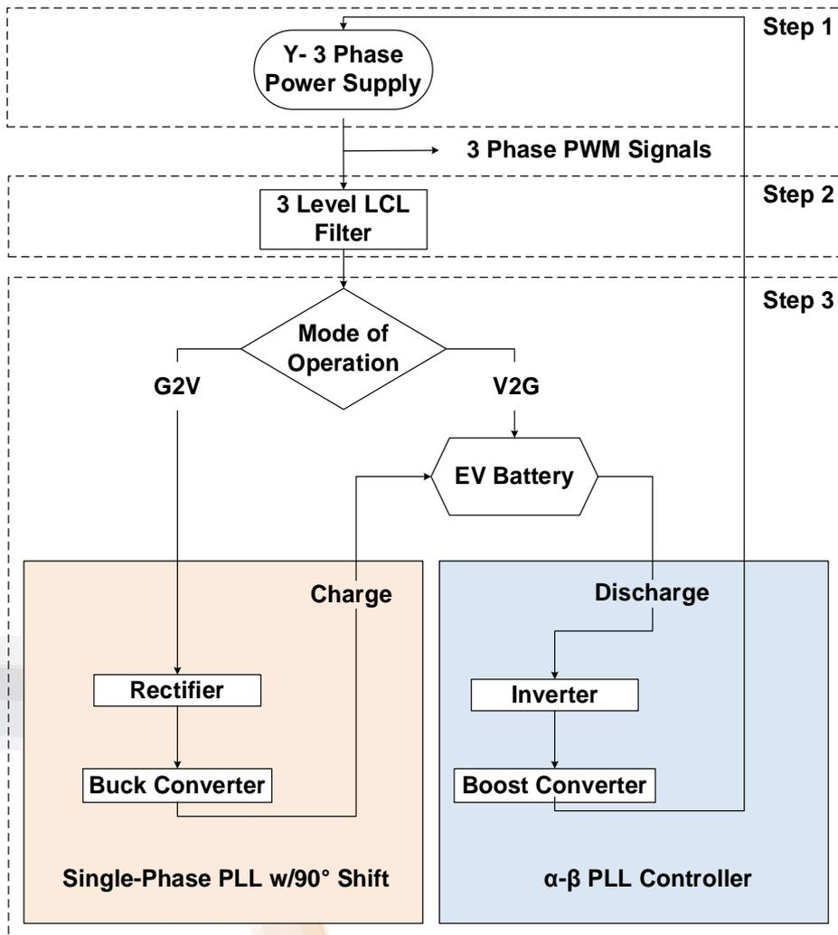
□ The operational mode, is determined by an input that tailors the PWM pulse signals for the switches accordingly.
