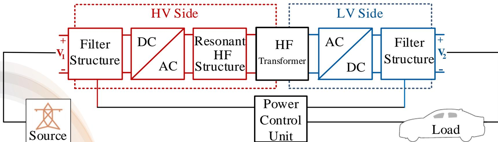
Figure: Block diagram of the basic structures in an isolated bidirectional DC/DC converter
