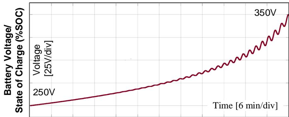
Figure. Simulink G2V Voltage Output
