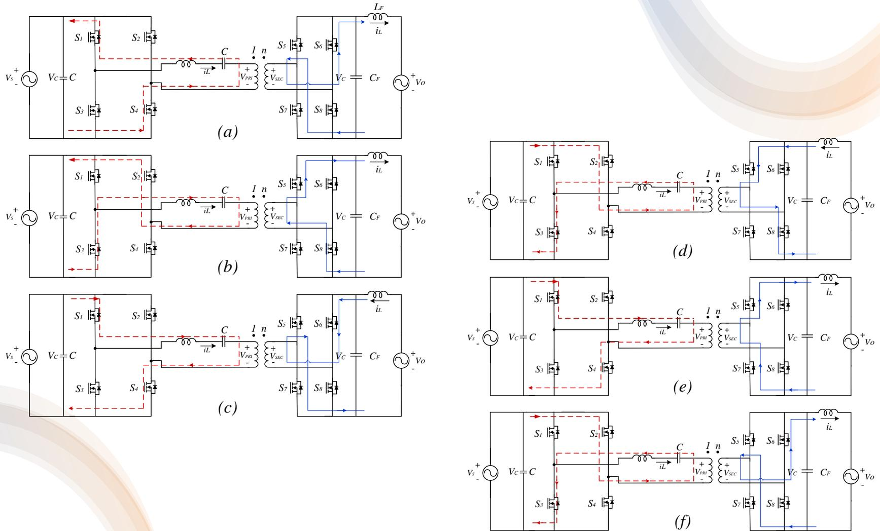
Figure. Operating phases of the DAB converter - Phases 1-6 (a-f)
