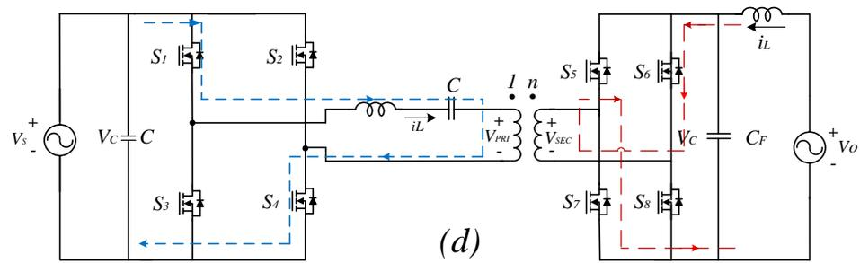
Figure d. V2G/Reverse Charging Mode of Operation
