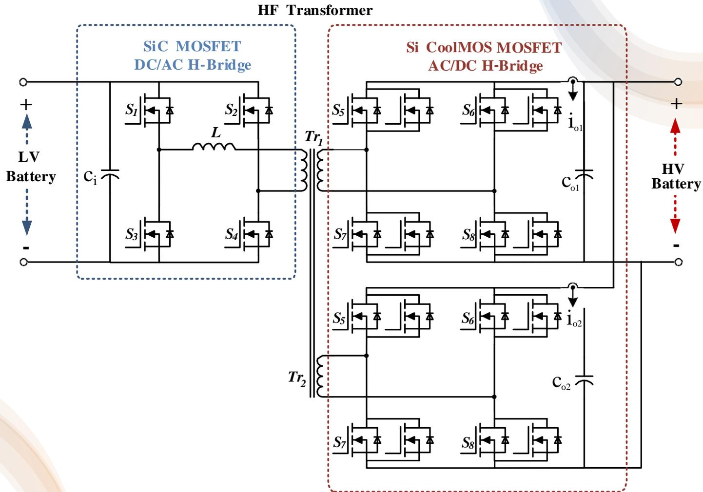
Figure. Main circuit diagram of the 5.6 kW DAB converter.
