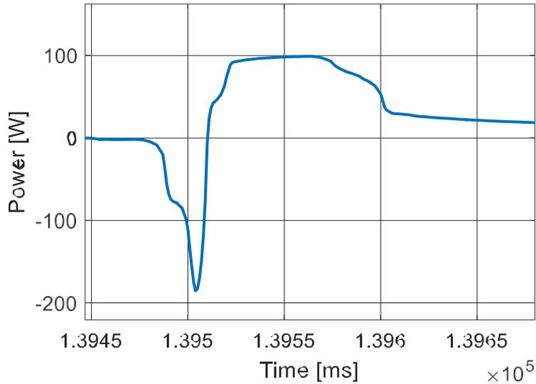
*Simulation Result for Switching Loss During Conduction for the Output H-Bridge Silicon Switches.*
