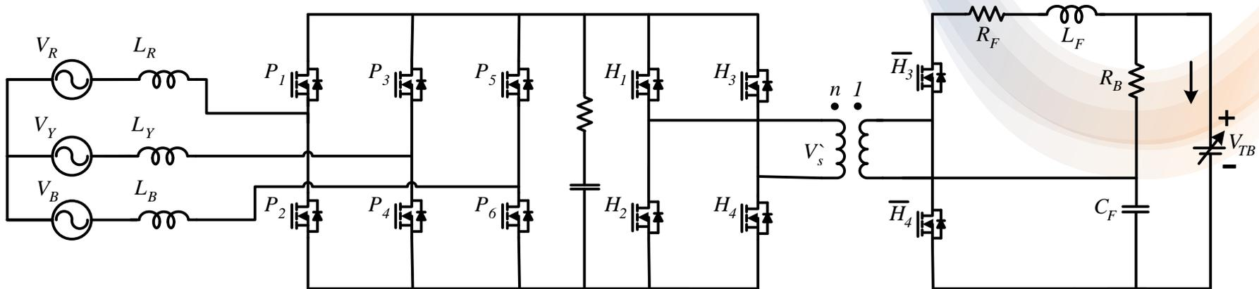
*Figure. AC-DC-DC Bidirectional Two-Stage Converter with V2G Capability*
