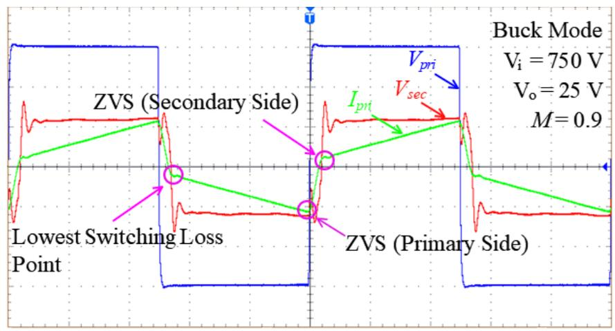
*Transformer Primary Voltage, Current, and Inductor Current Waveform*
