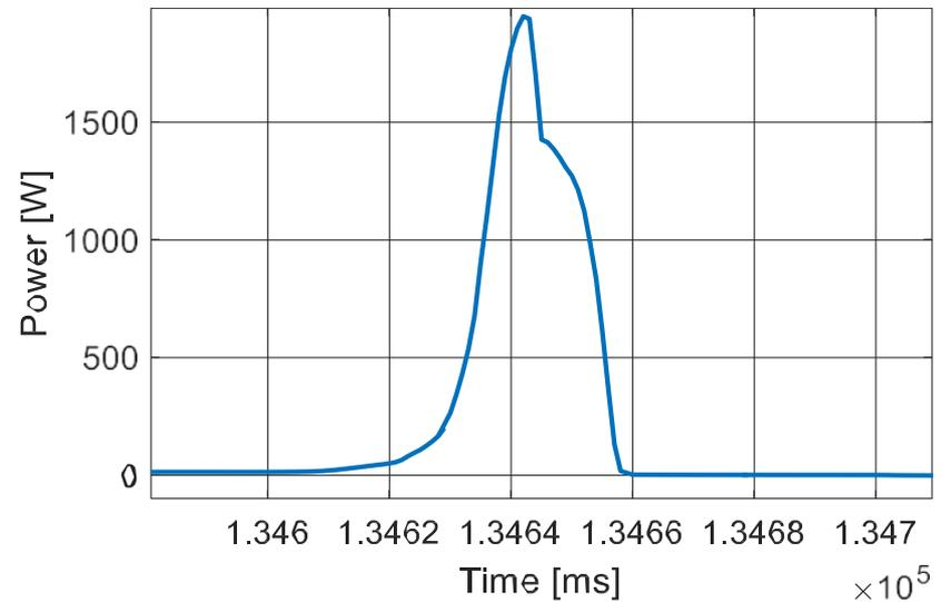
*Simulation Result for Switching Loss During Turn-Off for the Output H-Bridge Silicon Switches.*
