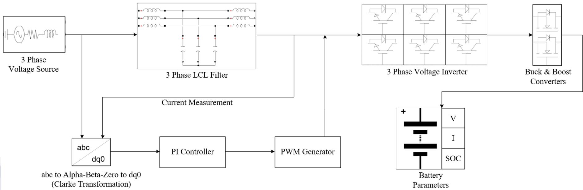
*Figure: Flow Chart Representation of the Simulation*
